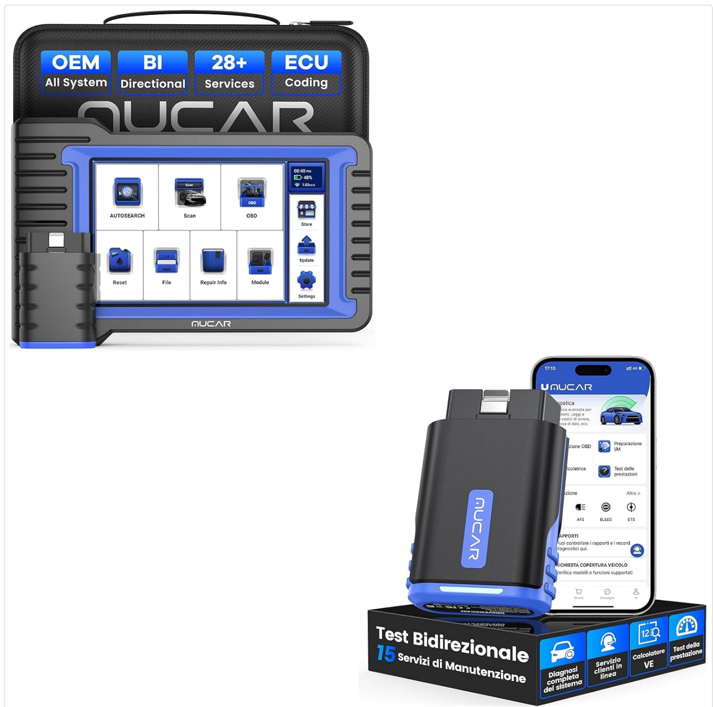
Figure 3.1: MUCAR VO7+ Drivescan OBD2 Scanner Diagnostic Tool. This image shows the main unit with its screen displaying the primary menu options like AutoSearch, Scan, OBD, Store, Update, Reset, File, Repair Info, Module, and Settings.
