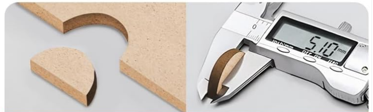
Cut 5mm MDF by one pass
