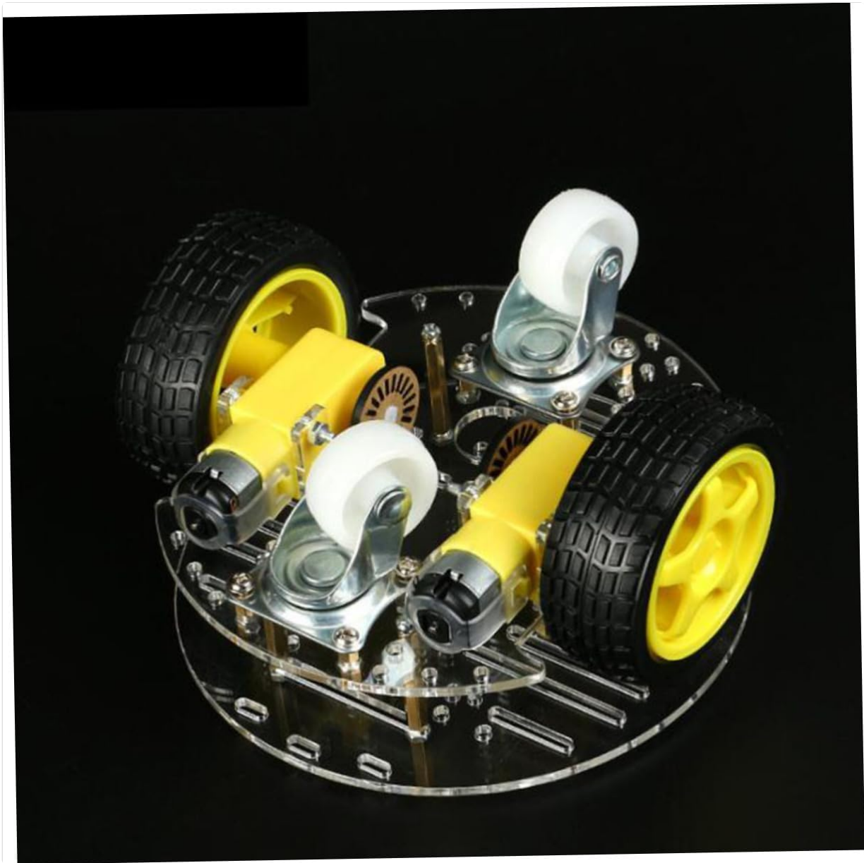
Image 4.2: Another view of the assembled chassis, highlighting the caster wheels for omnidirectional movement.
