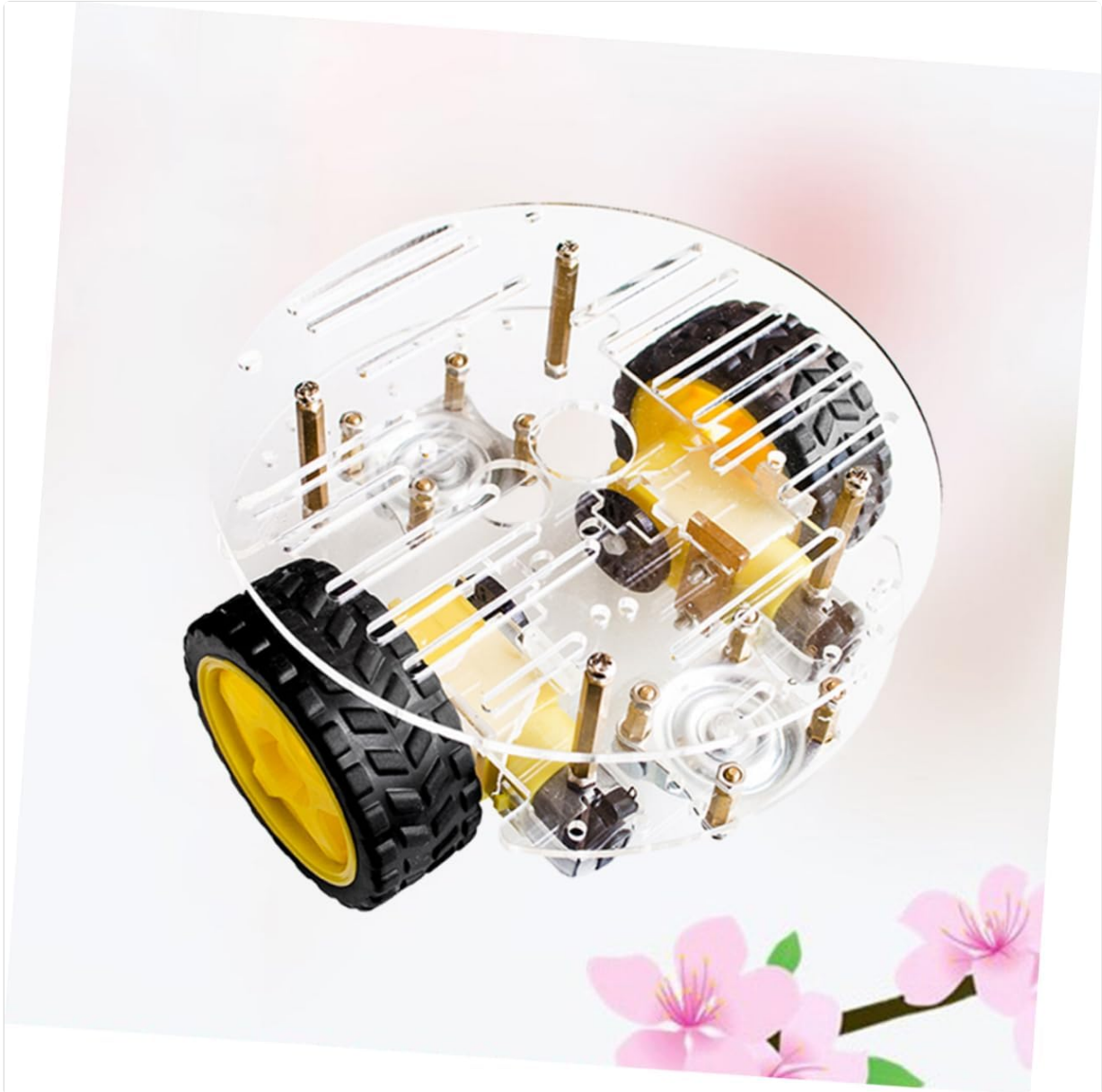
Image 4.1: Fully assembled OFFIGAM Smart Car Kit chassis, showcasing the double-layer design and motor/wheel placement.
