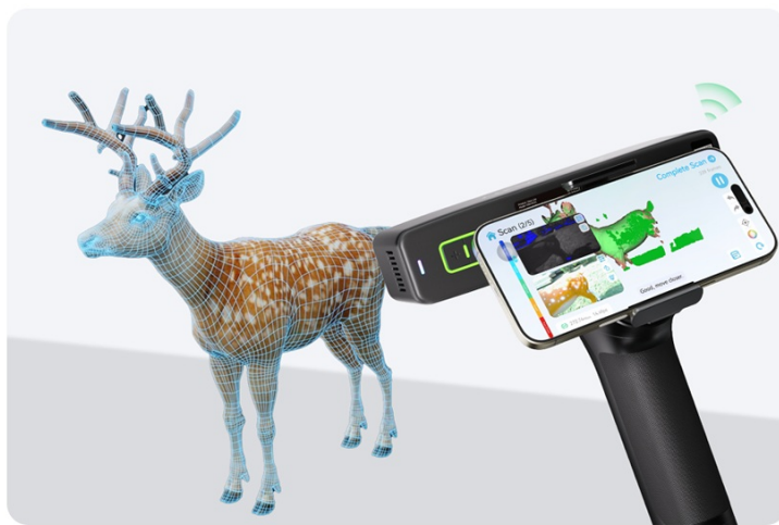
Figure 5.2: Using marker scanning for objects with limited features.
