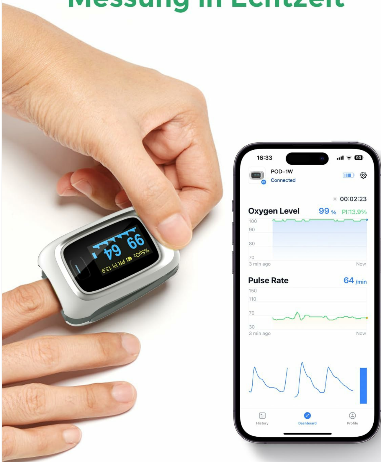
Image 6.1: A user demonstrating how to place a finger into the oximeter for a real-time measurement, with the accompanying app showing the live data feed.
