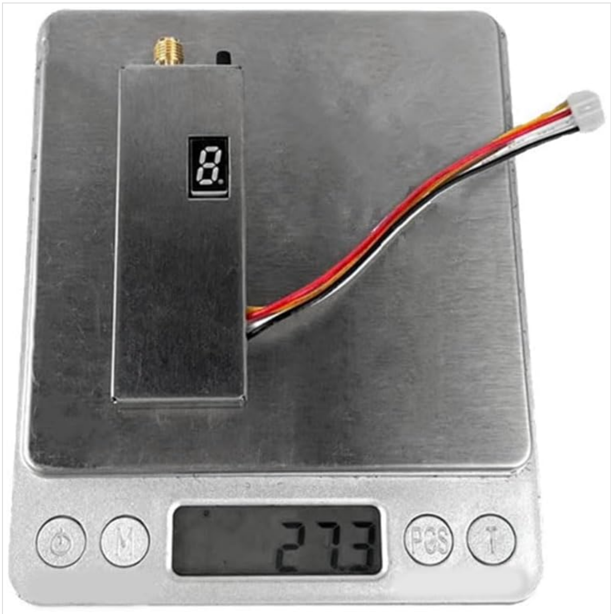
Figure 5.2: The transmitter unit being weighed on a digital scale, showing a weight of 27.3 grams.
