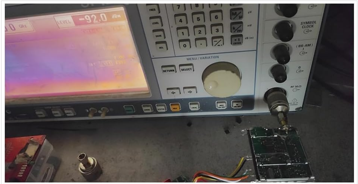
Figure 5.1: A test setup demonstrating the receiver's sensitivity, showing a reading of -92.0 dBm on a spectrum analyzer.
