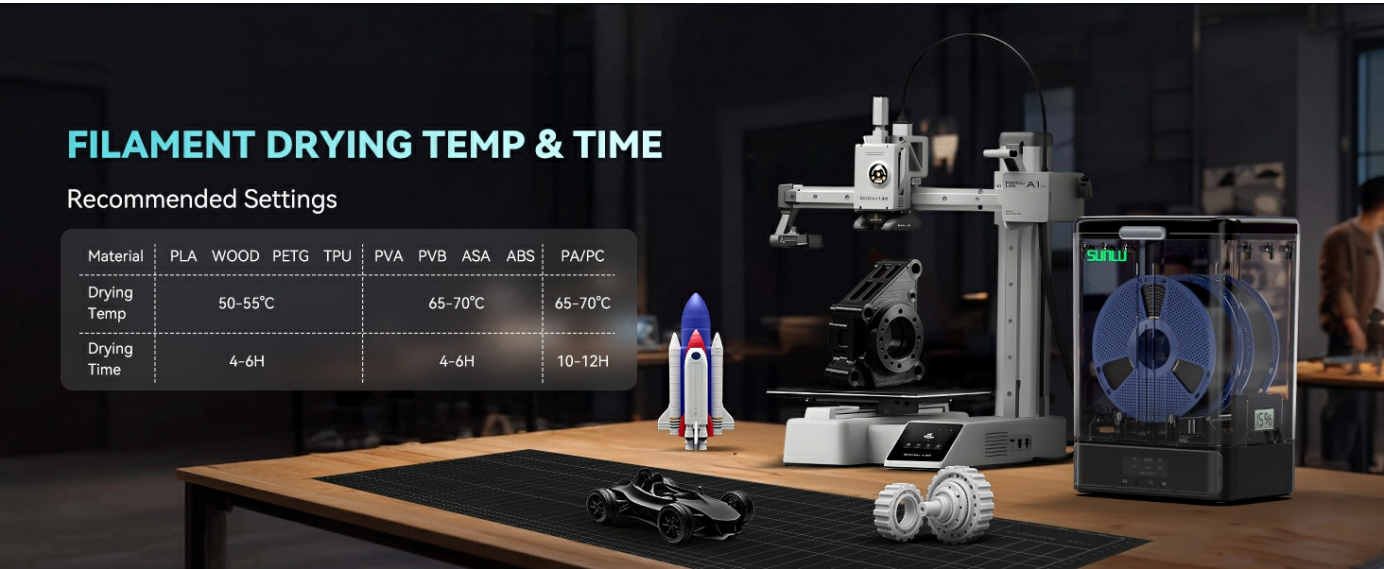
Image 6.2: Recommended Filament Drying Temperatures and Times.
