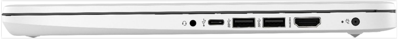
Figure 3.1: Right side of the laptop with power port, USB-A ports, USB-C port, HDMI port, and headphone jack.
