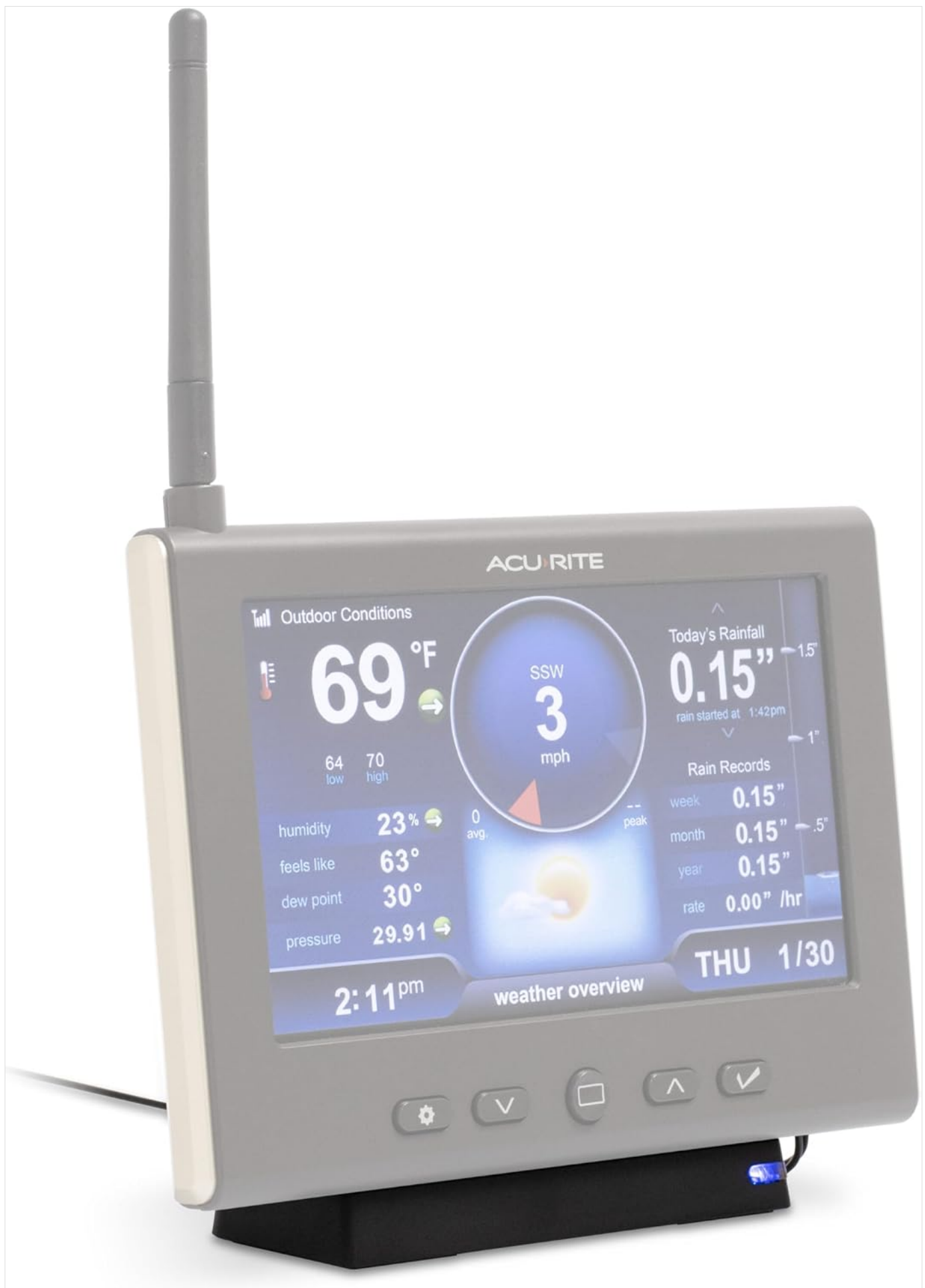
Image: An AcuRite HD display is shown docked into the power base, with the blue LED indicator light visible on the front, indicating normal operation or charging status.
