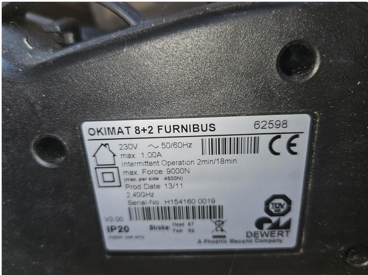
Image 2: Product label displaying model, electrical, and operational specifications.
