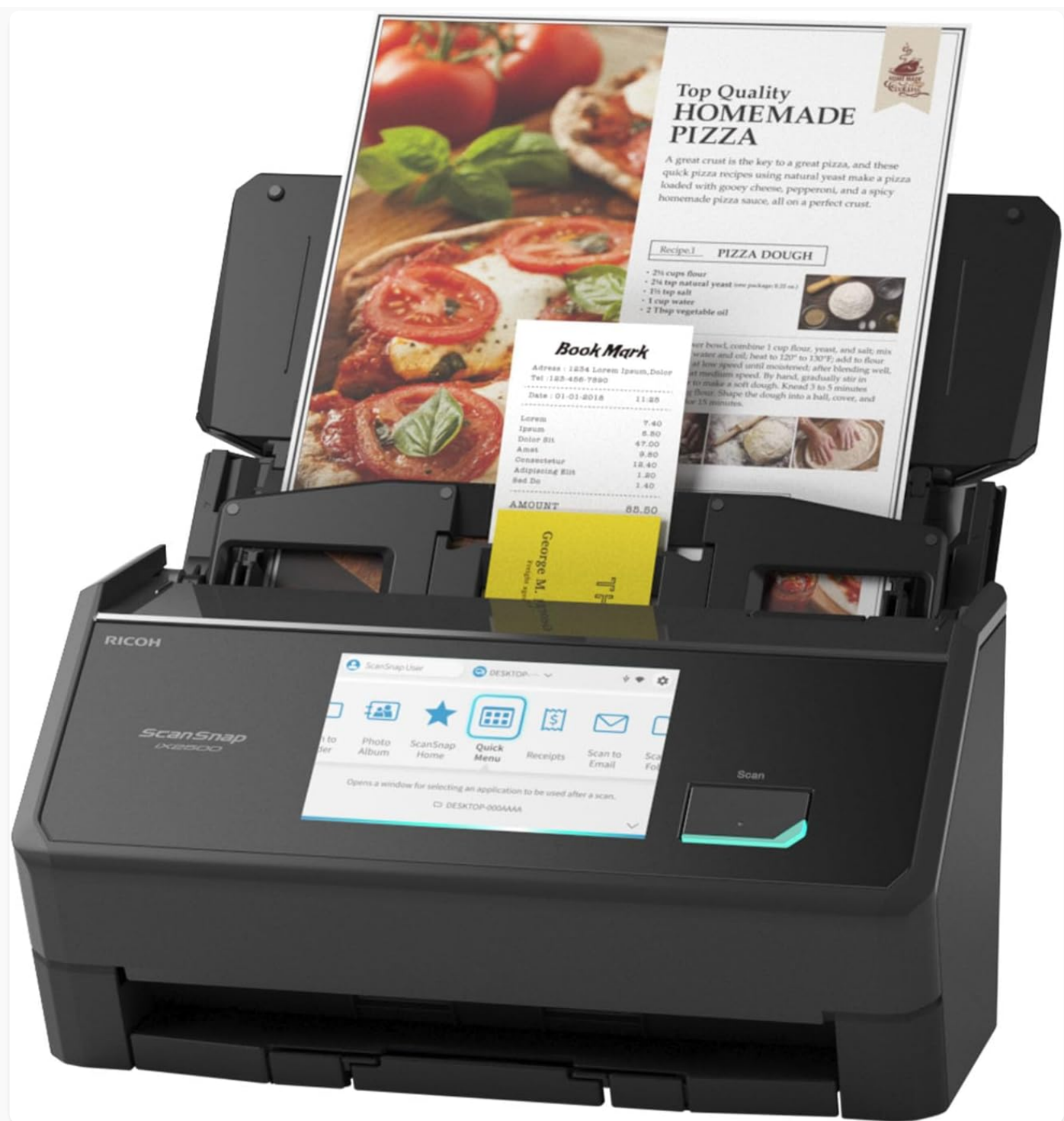
Figure 1.1: ScanSnap iX2500 Wireless Document Scanner in operation, scanning a document and a receipt.
