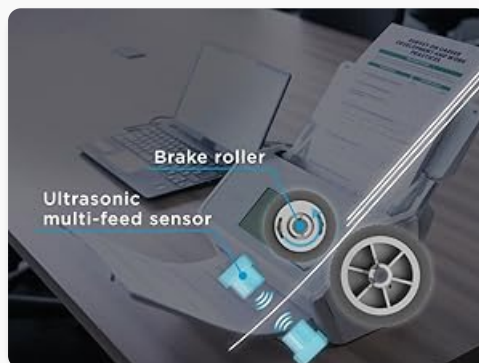
Figure 6.1: Internal mechanisms for smooth paper feeding and jam prevention.
