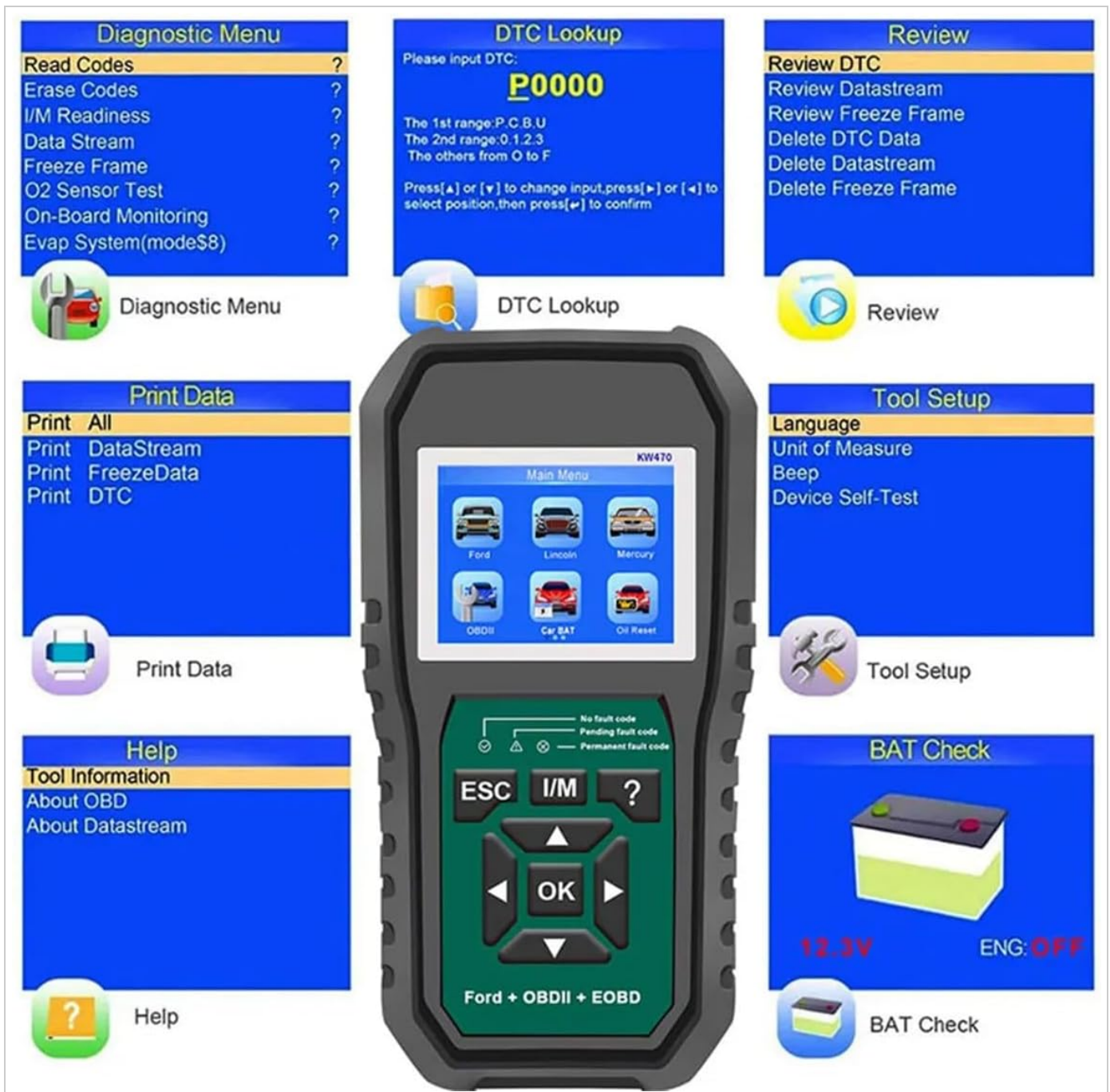
Figure 2.2: Overview of various diagnostic and utility menus available on the KW470 scanner.
