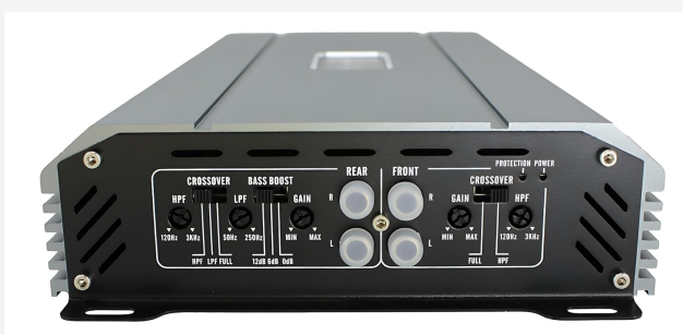
Figure 3: Control Panel. This image details the various controls on the amplifier, including Crossover (HPF, LPF), Bass Boost, and Gain adjustments for both front and rear channels. It also shows the Protection and Power indicator lights.
