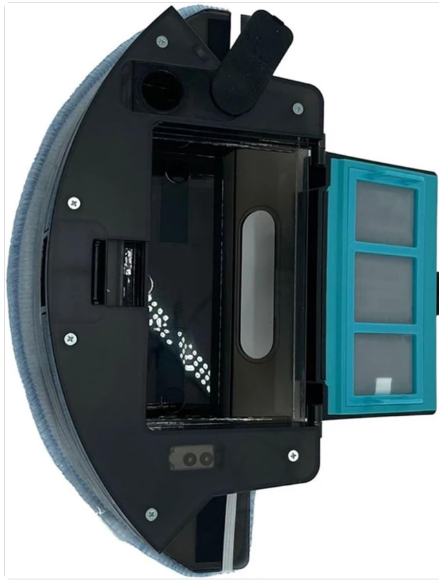
Figure 5.1: Angled view of the tank, useful for understanding filter access for cleaning.
