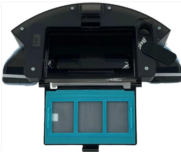
Figure 4.1: Top view of the tank with compartments open, revealing the filter and internal structure.
