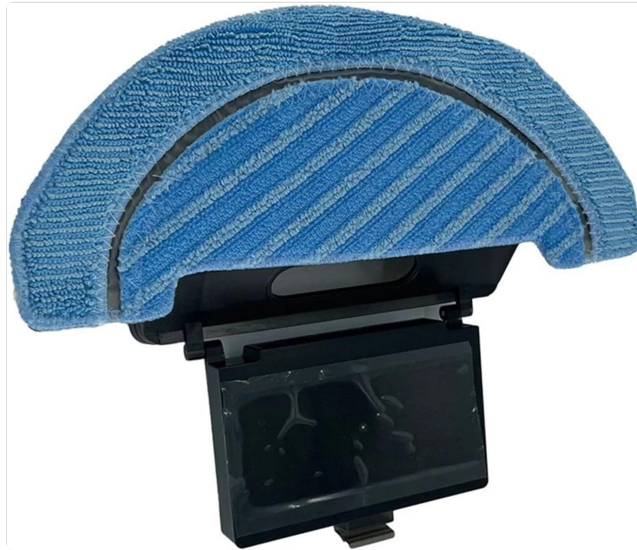
Figure 4.4: Bottom view of the tank, highlighting the integrated mop pad.
