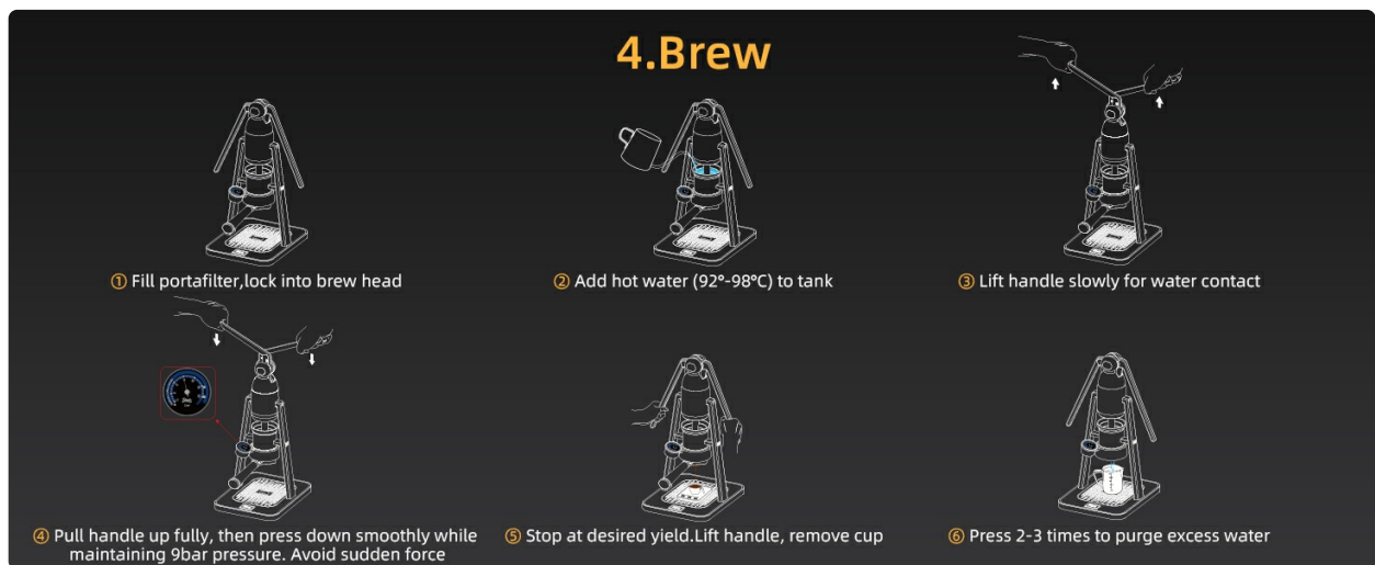
Image: A visual breakdown of the brewing process, from filling the portafilter to final extraction and purging.
