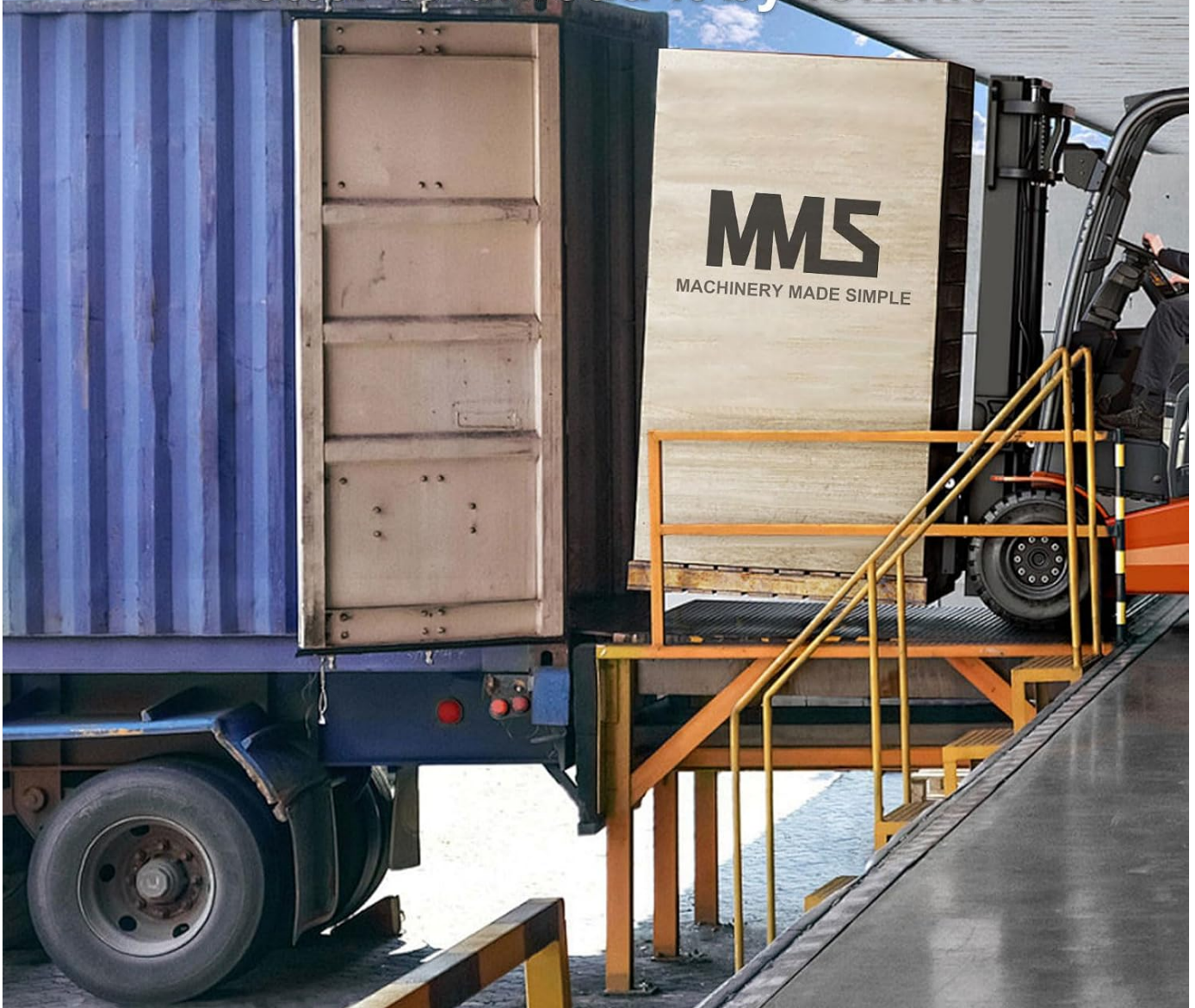
Figure 5: Unloading the Skid Steer. This image demonstrates the recommended method for safely unloading the crated machine using a forklift.
