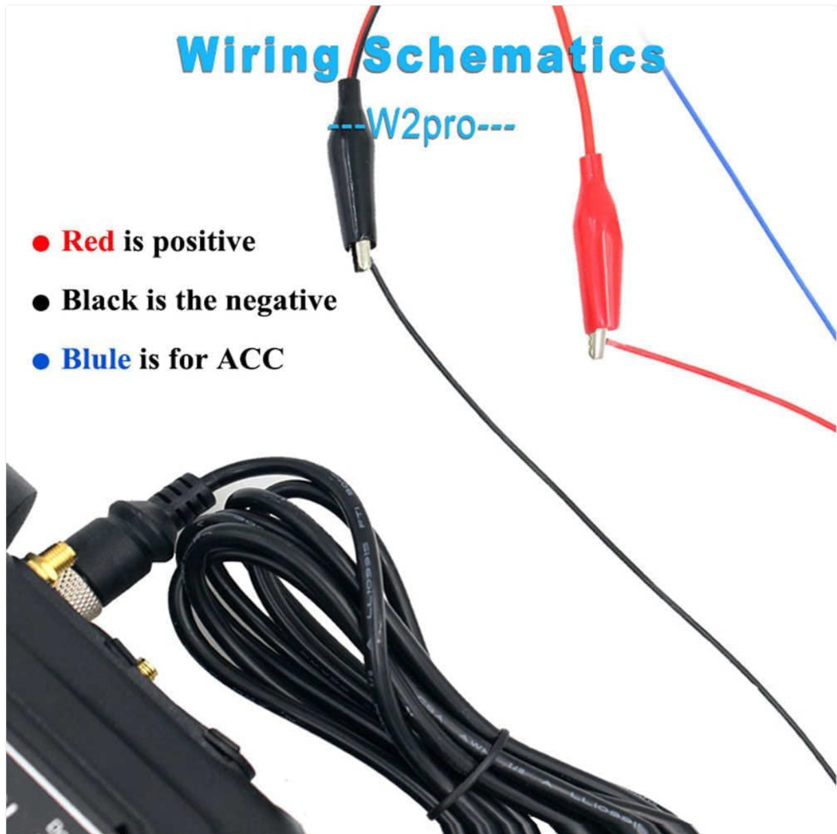
Image 3.1: Wiring schematics for the ANYSECU W2 Pro. The red wire is for positive power, the black wire is for negative/ground, and the blue wire is for ACC (Accessory) power, typically connected to the vehicle's ignition switch.
