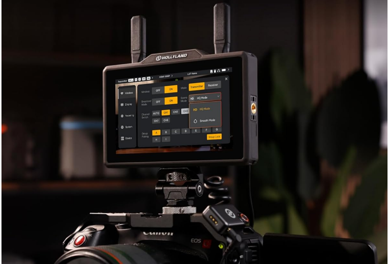
Figure 5.1: Select between HD Mode for clarity or Smooth Mode for lowest latency.
