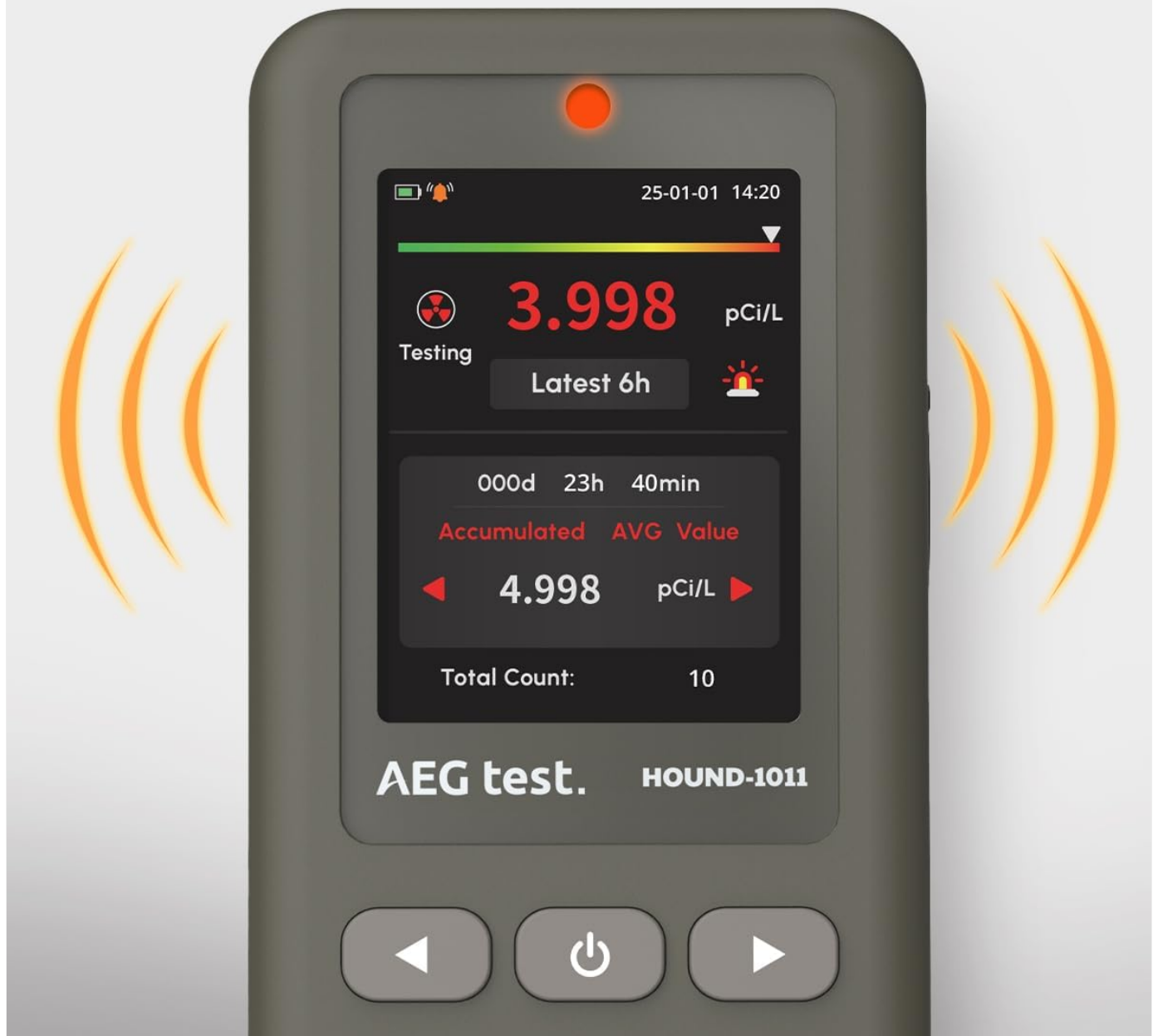
Image 4.4: The HOUND-1011 display indicating an alarm condition due to elevated radon levels.
