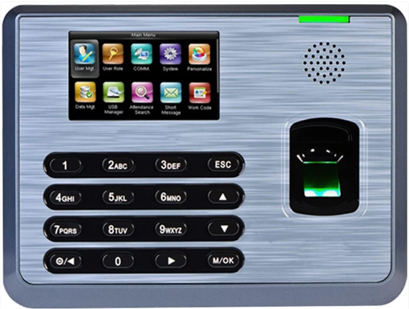
Figure 2.2.1: Front View of the TX628-WIFI Device. This image displays the front panel of the time attendance system, featuring the color TFT screen, numerical keypad, function buttons, fingerprint scanner, and integrated speaker.
