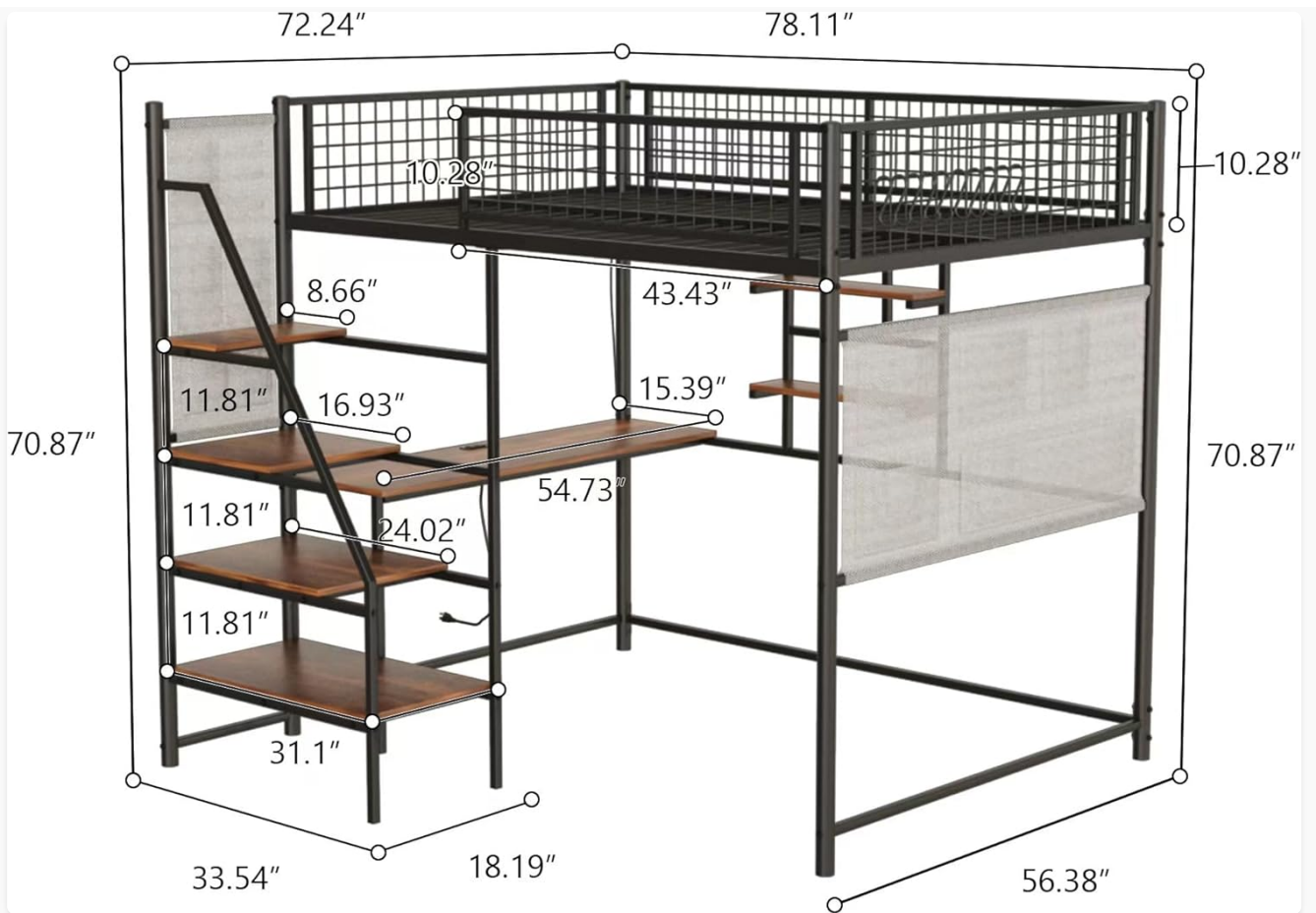
Image 4.1: Detailed dimensional diagram of the loft bed, useful for assembly and space planning.
