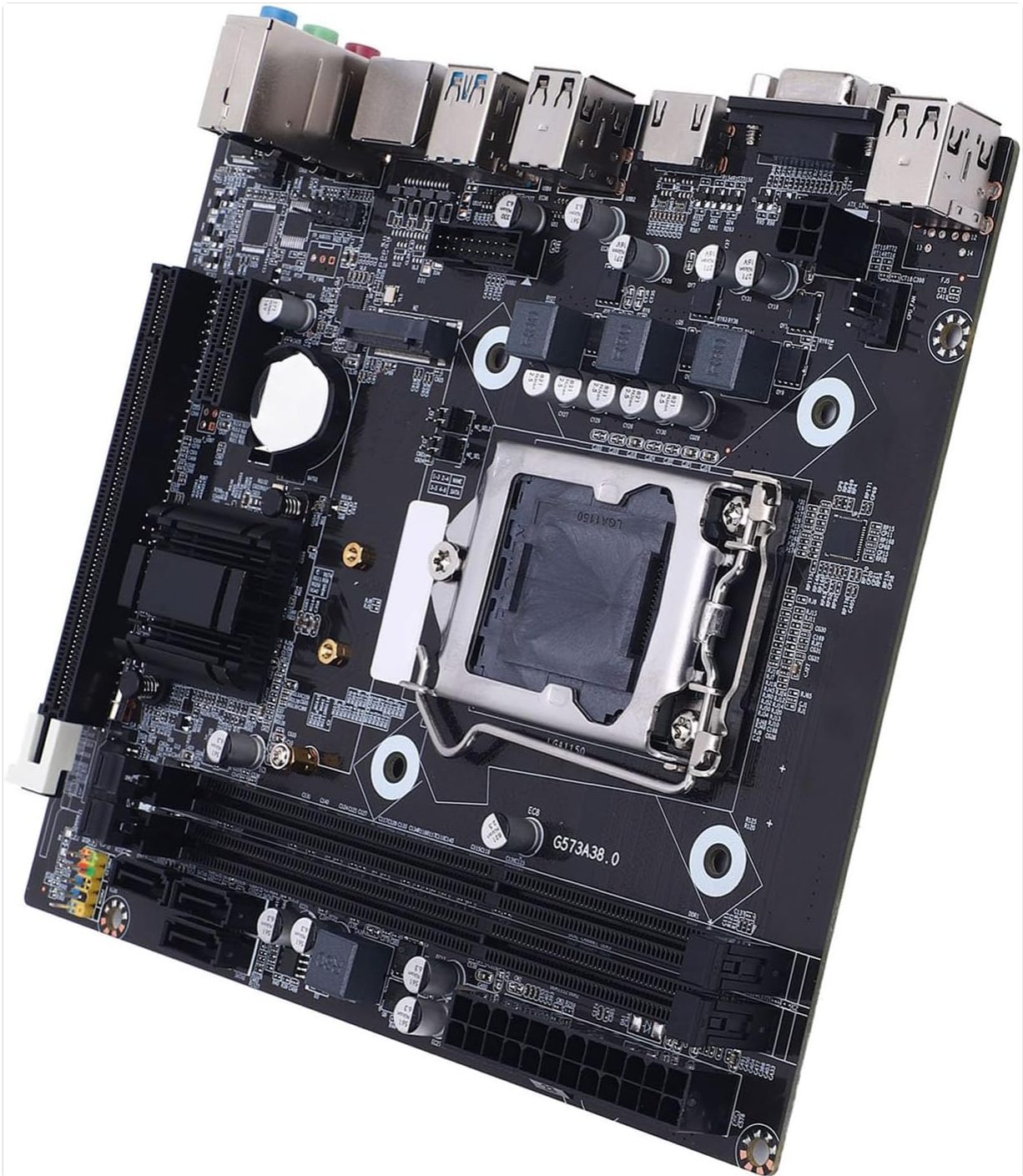
Figure 3.1: Front view of the Yoidesu H81 M-ATX LGA 1150 Motherboard, showing the CPU socket, RAM slots, and various connectors.
