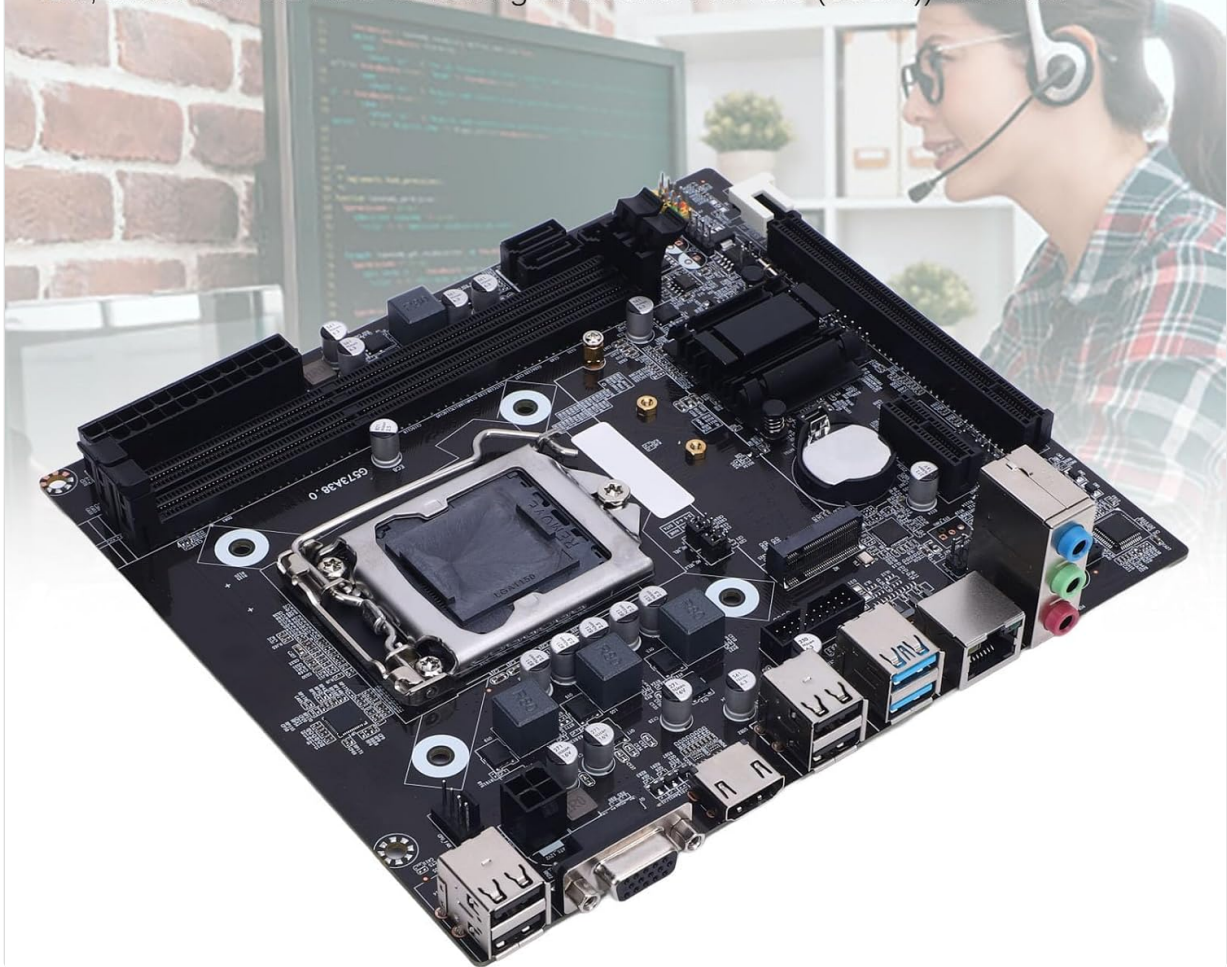
Figure 5.3: View of the high-speed M.2 interface on the Yoidesu H81 motherboard, indicating its support for both NVMe and NGFF drives via jumpers.
