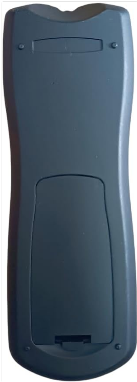
Figure 3: Back view of the remote control. This image shows the battery compartment cover.
