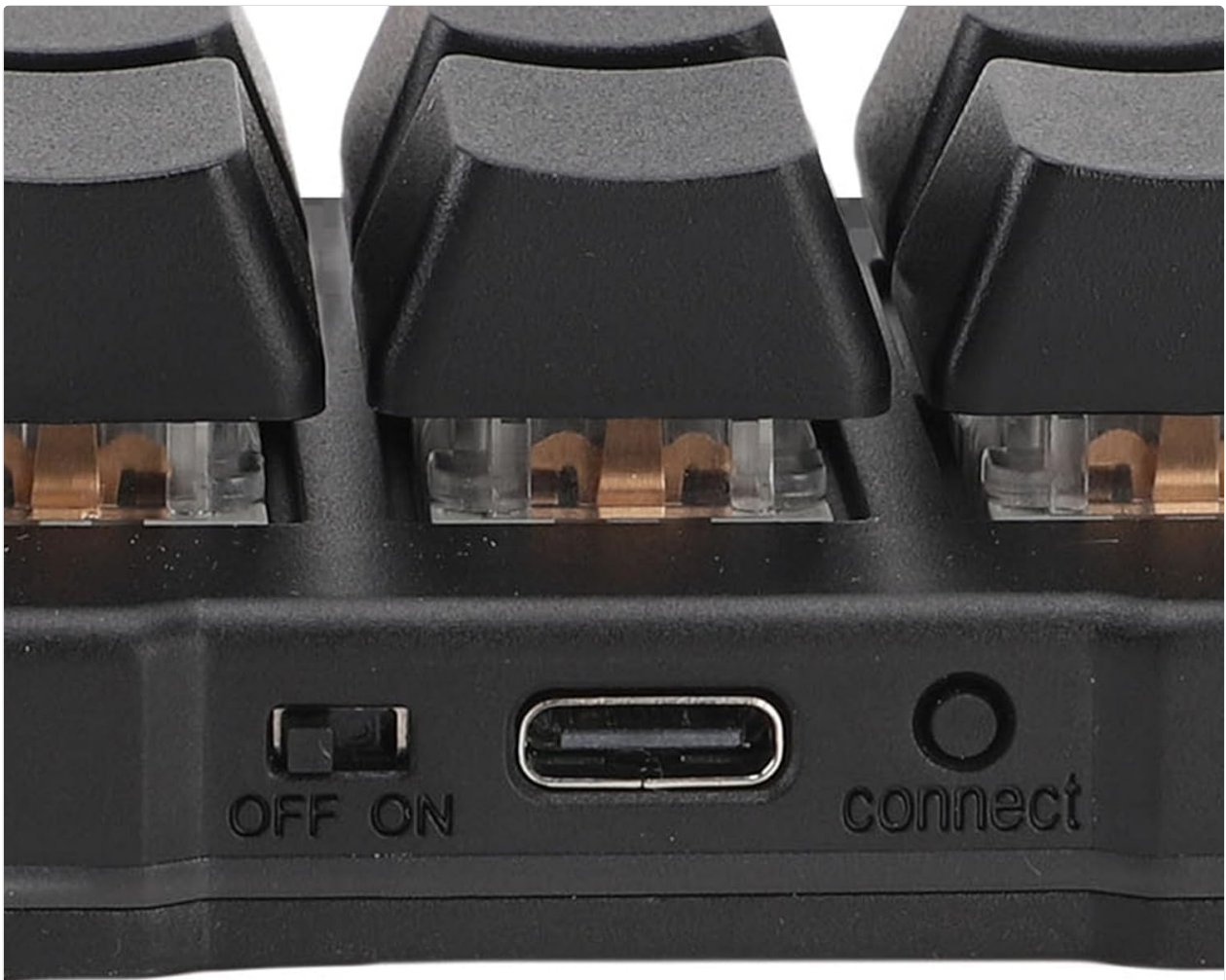
Figure 3: Detailed view of the keypad's side, featuring the power switch, USB Type-C port, and 'connect' button.
