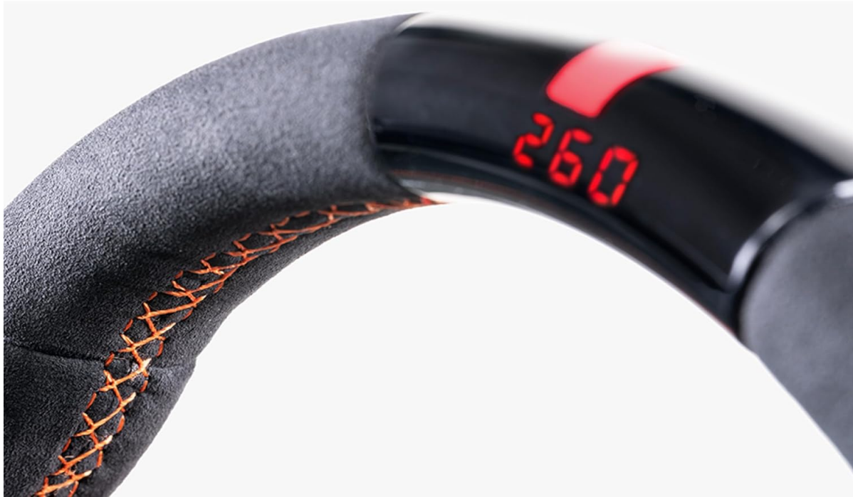
Image 4.2: The RevStripe LED display showing numerical data and RPM indication.
