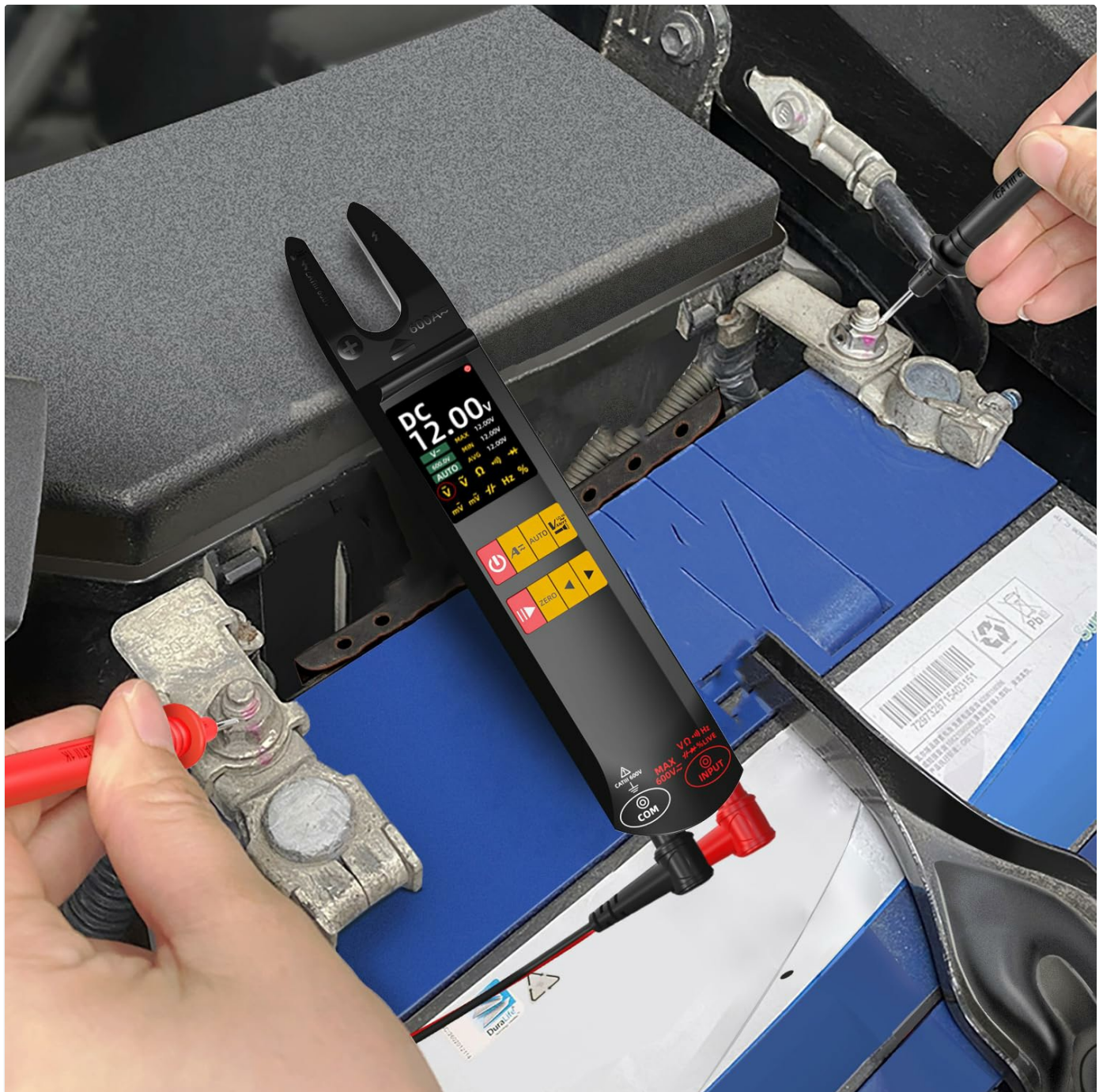
Figure 5: Measuring DC voltage on a battery.
