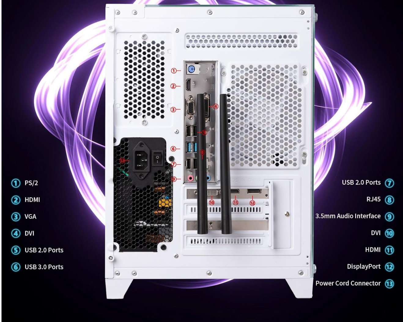
Image 3.1: Rear I/O ports of the abytespark Gaming PC. Note: Do not use the video ports on the motherboard (VGA, DVI, HDMI next to USB ports) if a dedicated graphics card is installed. Connect your monitor to the graphics card's ports (HDMI, DisplayPort, DVI located lower on the case).
