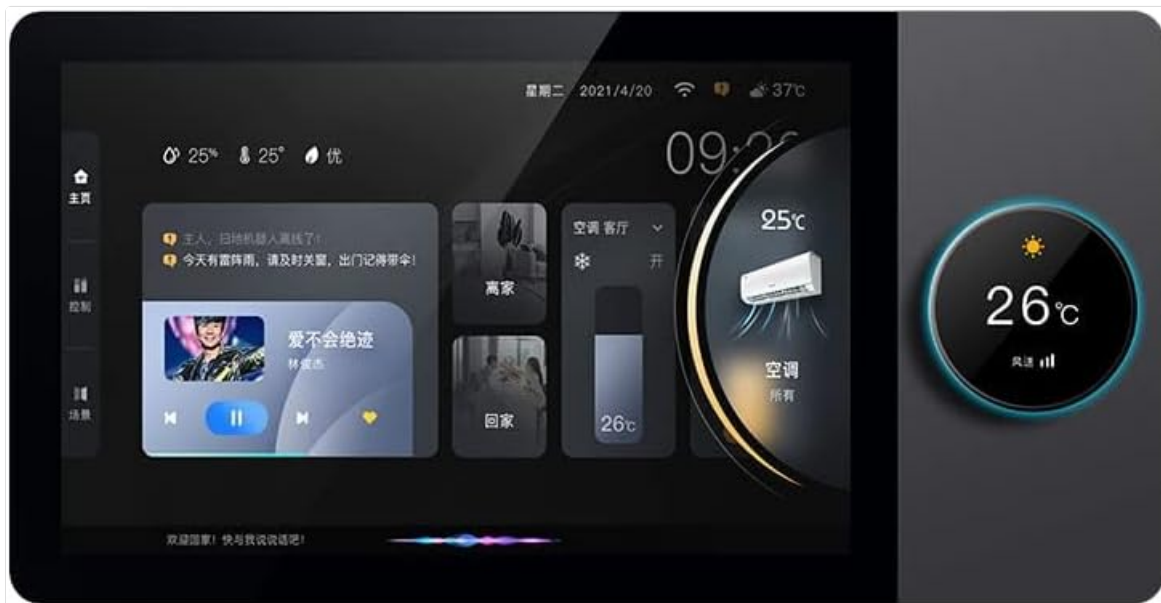
Figure 3: The main interface of the control panel, showing various smart home controls and a rotary switch on the side.
