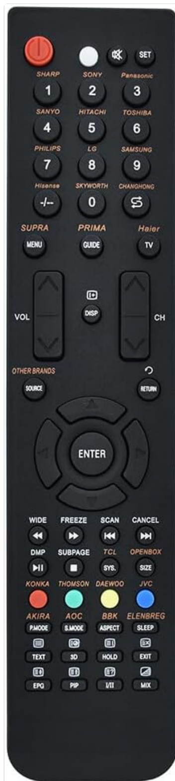
Image: Front view of the remote control, displaying the layout of all buttons, including dedicated brand keys for programming.
