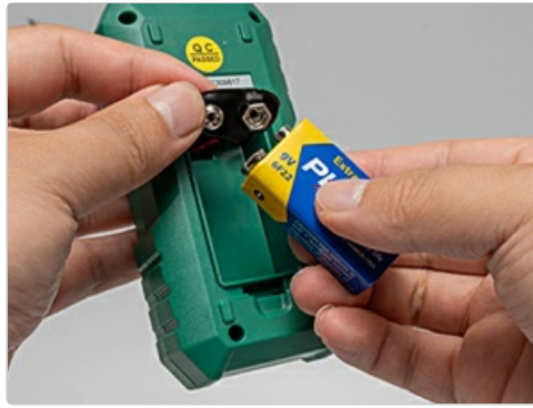
Image 5.1: Proper installation of the 9V battery.
