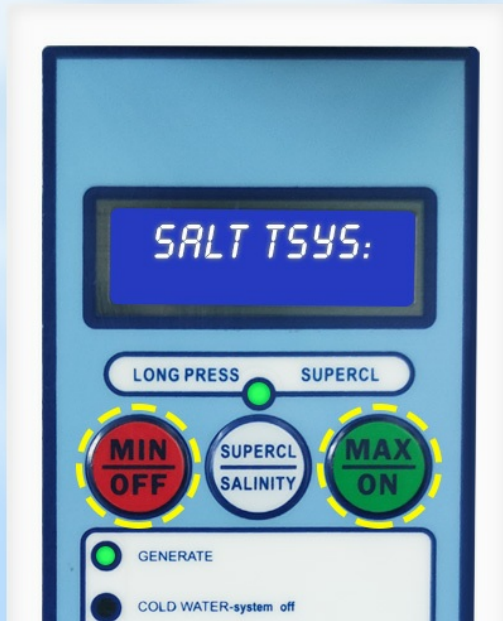
Image 5.2: Salinity calibration procedure.
