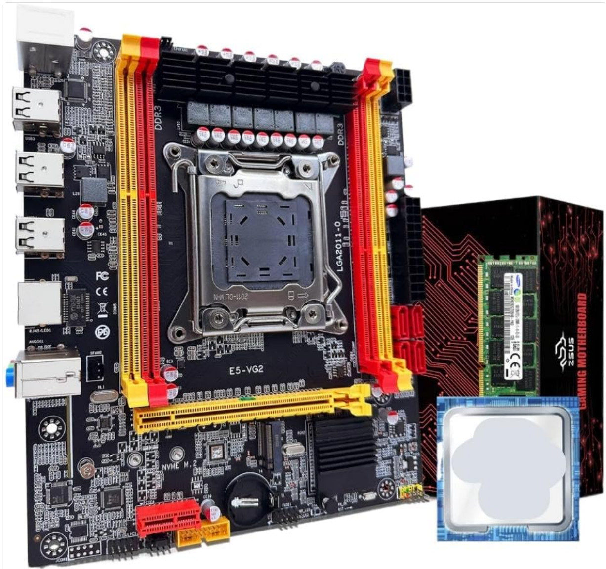
Figure 1: ZSUS X79 VG2 Motherboard Bundle. This image displays the motherboard with its LGA2011 CPU socket, four DDR3 RAM slots, PCIe slots, and various connectors. The included Xeon E5 2689 C2 CPU and 16GB DDR3 ECC RAM module are also visible alongside the product packaging.
