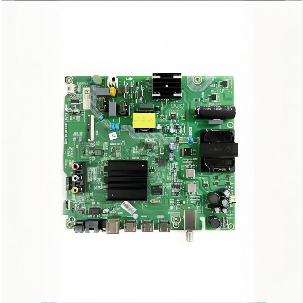
Figure 2: Detailed view of the input/output interfaces on the RSAG7.820.9746 motherboard. This close-up highlights the HDMI ports, USB ports, and the red, white, and yellow RCA (AV) input jacks, along with associated circuitry and a heat sink.
