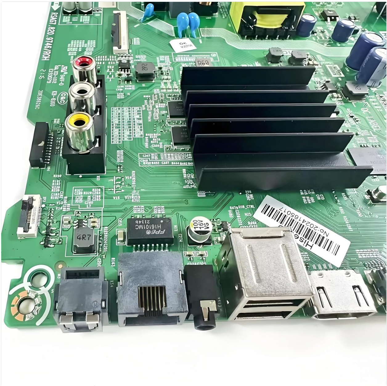
Figure 3: Angled view of the RSAG7.820.9746 motherboard, showing the arrangement of connectors and components. This perspective helps in identifying specific connection points during installation.
