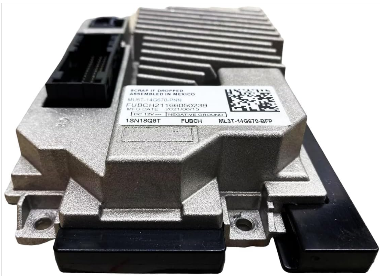
Image 5.2: Side view of the SYNC4 APIM NAV Module, showing the heat dissipation fins and identification label.
