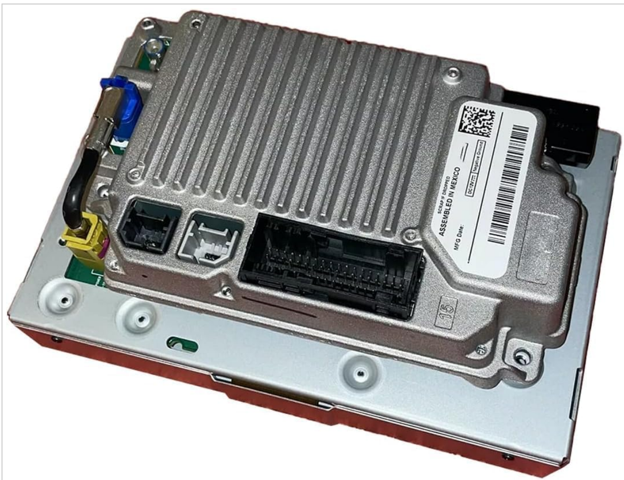
Image 5.1: Rear view of the SYNC4 APIM NAV Module, illustrating the primary electrical and antenna connections.
