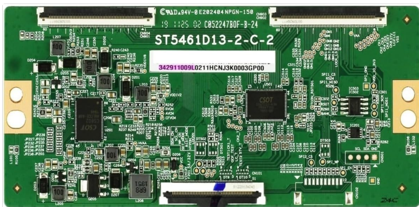
Figure 1: RXCWWZQQ 342911009L ST5461D13-2-C-2 T-con Logic Board. This image shows the top view of the T-con board, highlighting its various components and connectors.
