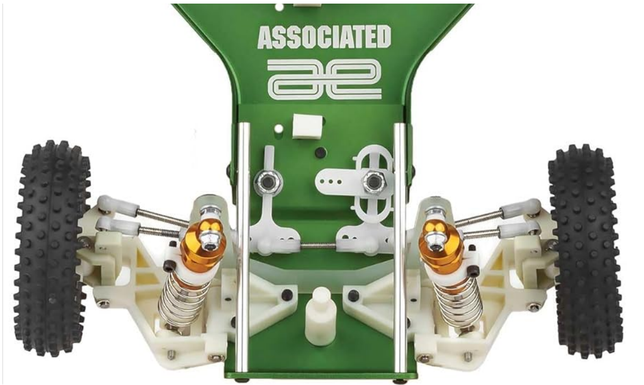
Image: A top-down view of the RC10 Green Masters Edition chassis, highlighting the green monocoque tub and suspension components.
