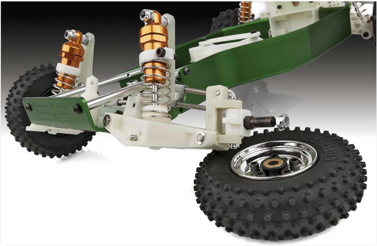
Image: A detailed view of the front suspension and wheel assembly, showing the adjustable racing shocks and steering components.
