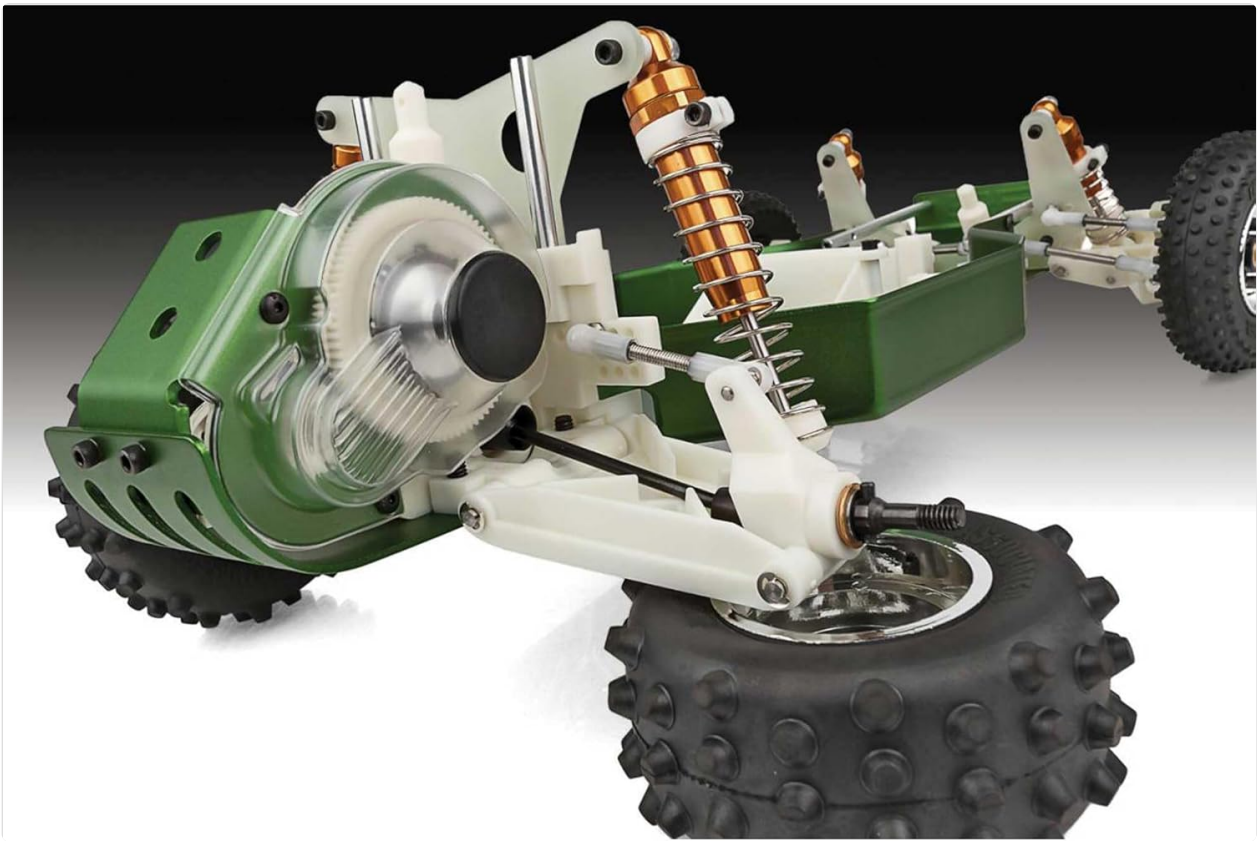
Image: A detailed view of the rear suspension and drivetrain, showing the motor mount area and adjustable shocks.
