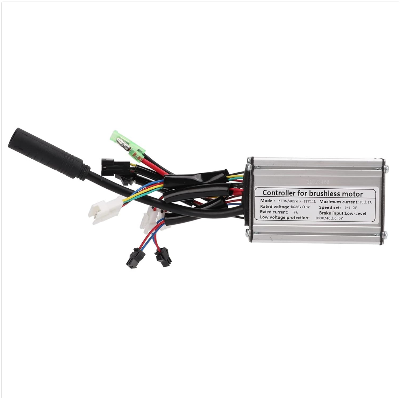
Figure 3.1: Overview of the plplaaoo 15A Sine Wave Controller with its connected wiring harness.
