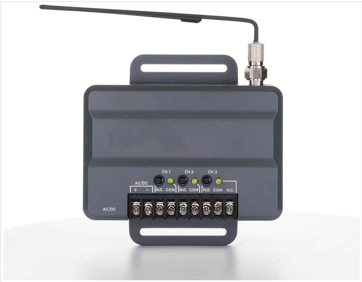
Figure 1: Anderic RR850LM Universal Receiver unit showing AC/DC power input and three channels (CH.1, CH.2, CH.3) with Normally Open (N.O.), Common (COM), and Normally Closed (N.C.) terminals. The receiver unit features clearly labeled terminals for AC/DC power input and three distinct channels for connecting to gate or garage door operators. Each channel provides Normally Open (N.O.), Common (COM), and Normally Closed (N.C.) connections.
