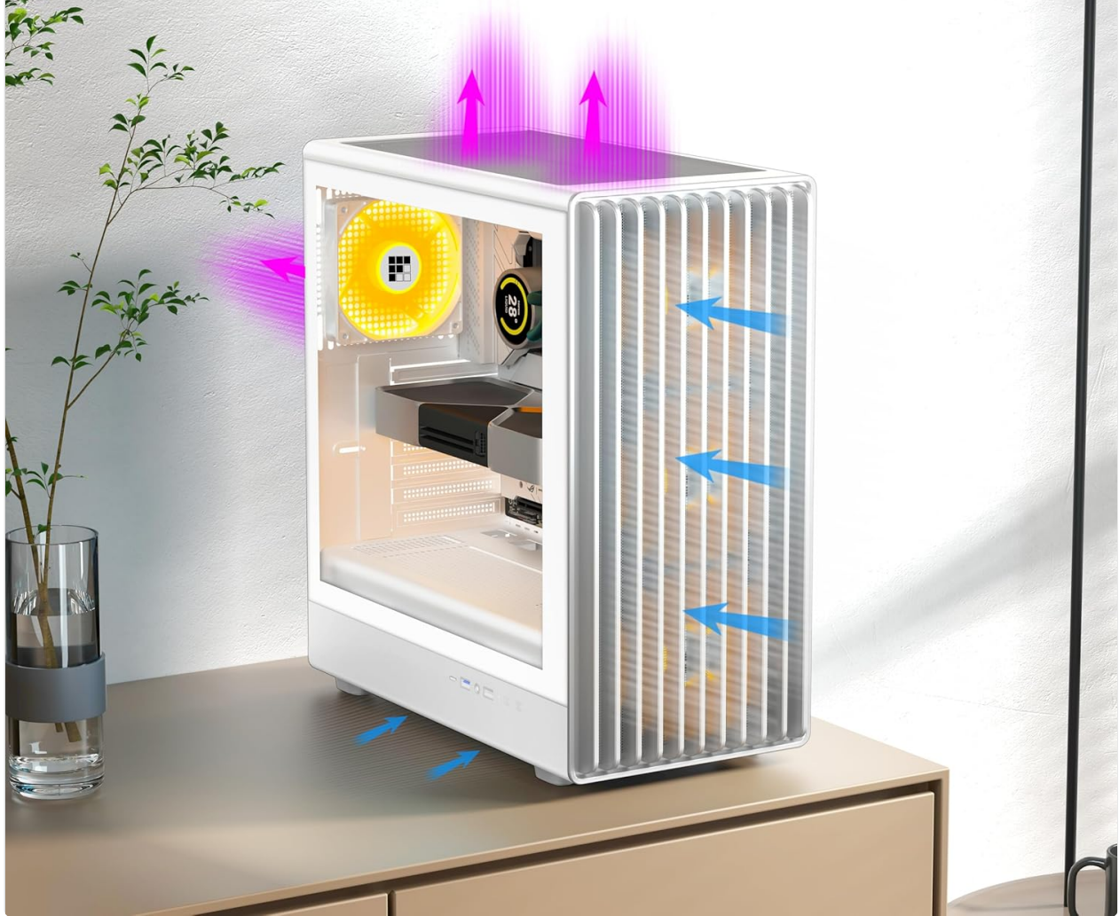
Image 2.4: Airflow optimization within the case, with cold air intake and hot air exhaust.
