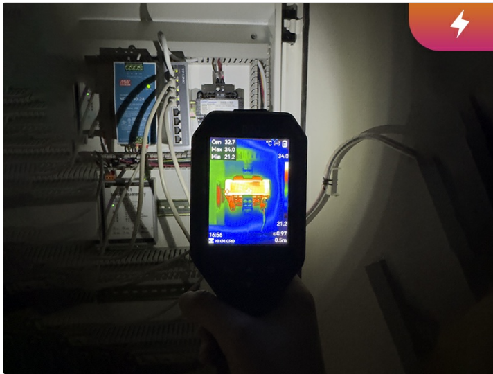
Figure 3.5: LED Work Light in Use. This image shows the B20's LED work light providing illumination in a low-light environment, aiding visual inspection.
