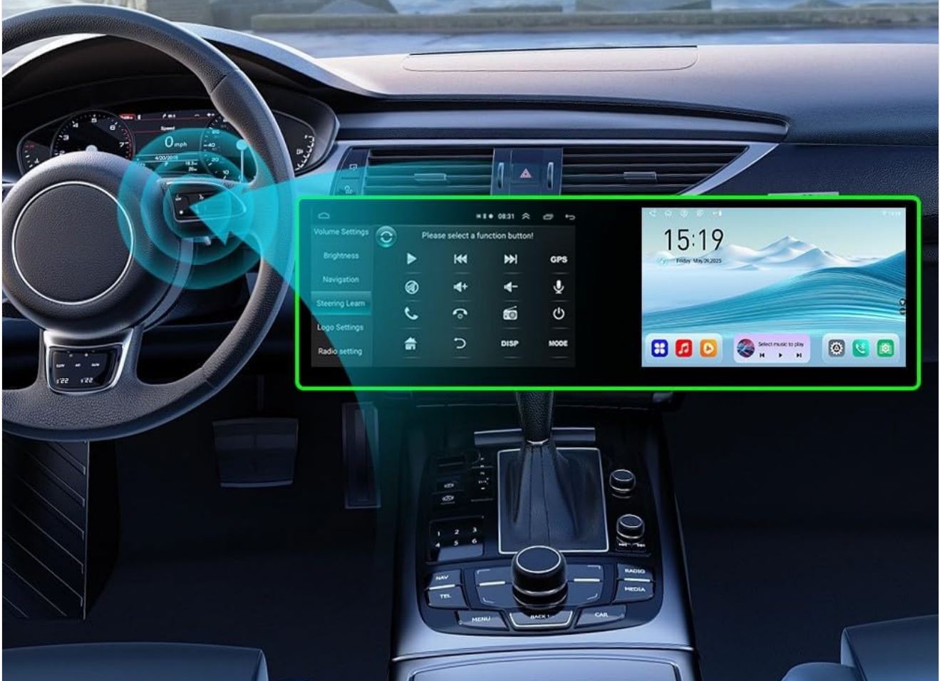
Figure 5: Steering Wheel Control. The image demonstrates how the head unit integrates with vehicle steering wheel controls, allowing drivers to manage audio and settings without taking their hands off the wheel.
