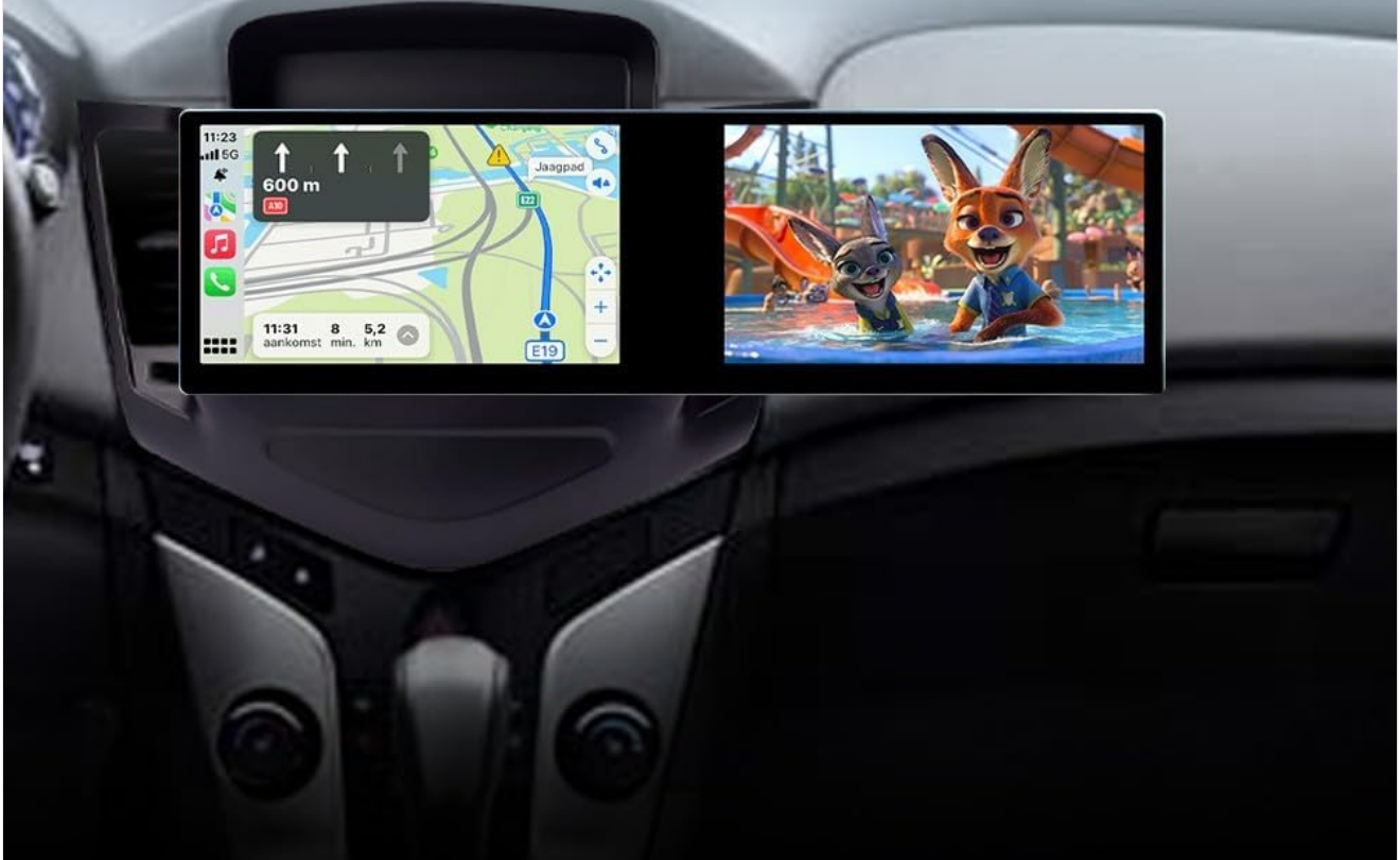
Figure 4: Dual Screen Display. This image illustrates the head unit's ability to display two different applications concurrently, such as a navigation map and a video player.
