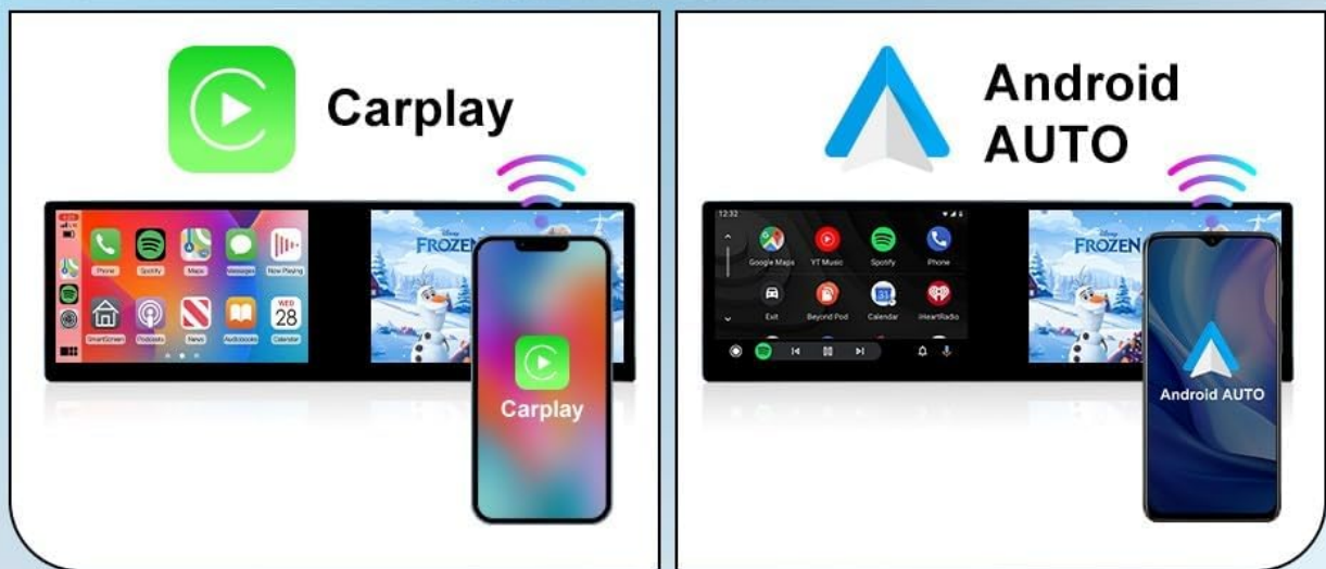
Figure 2: Wireless CarPlay/Android Auto. This image illustrates the integration of smartphone interfaces (CarPlay and Android Auto) onto the head unit, enabling access to navigation, music, and voice assistants like Siri.
