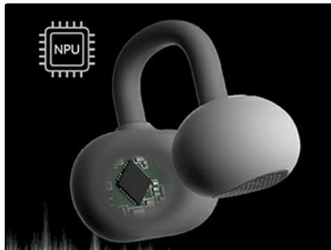
Image: A diagram highlighting the Neuron Processor Unit (NPU) chip integrated into the earbud, responsible for the AI Environmental Noise Cancellation (ENC) functionality.
