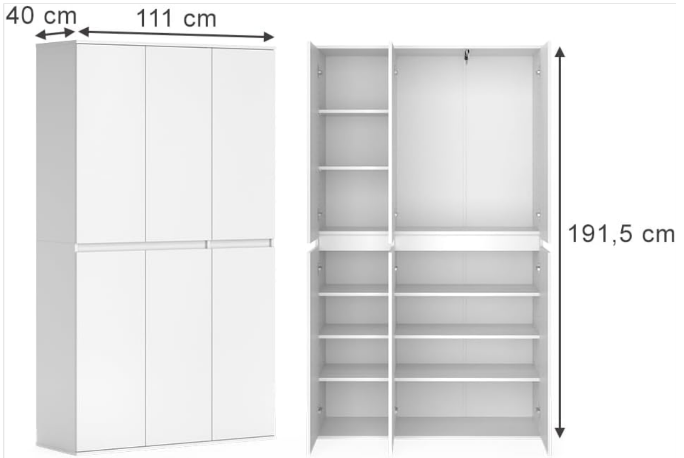
Figure 2: Dimensional diagram of the Vicco Claus Wardrobe. Overall dimensions are approximately 111 cm (width) x 40 cm (depth) x 191.5 cm (height).
