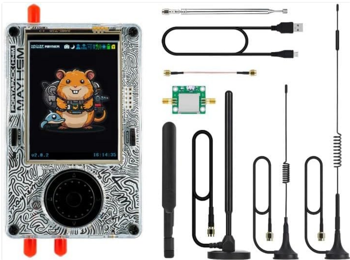
Image: Overview of the Celonix H4M PortaPack kit, showing the main unit, multiple antennas for different frequency ranges, an LNA, and a USB cable.
