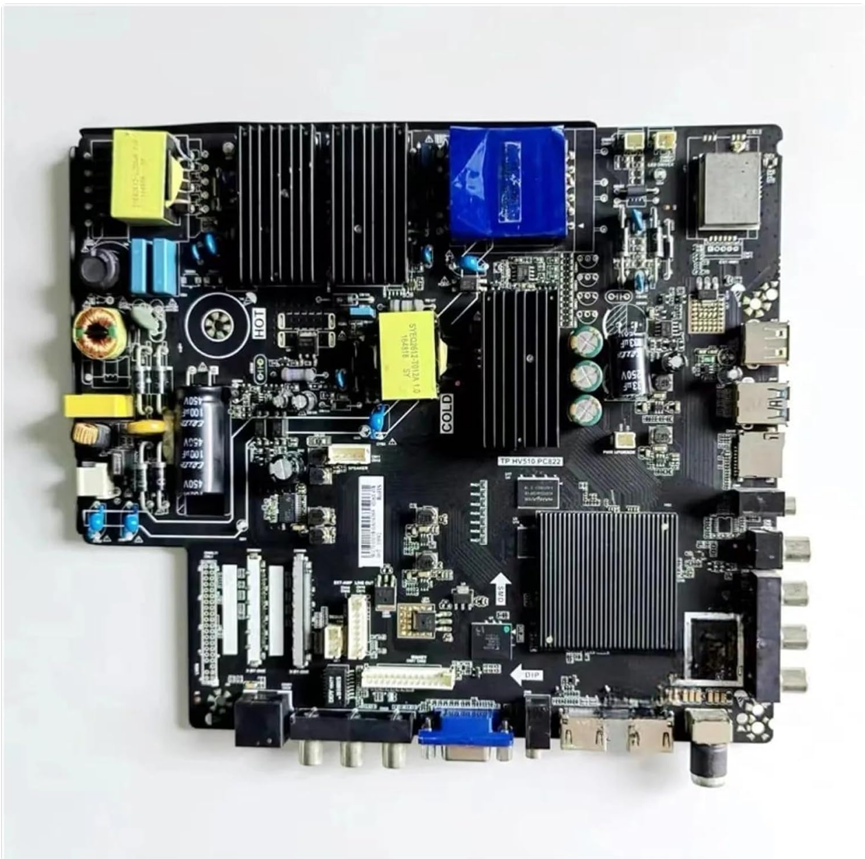
Figure 2.1: RIMBILIE TP.HV510.PC822 TV Motherboard
