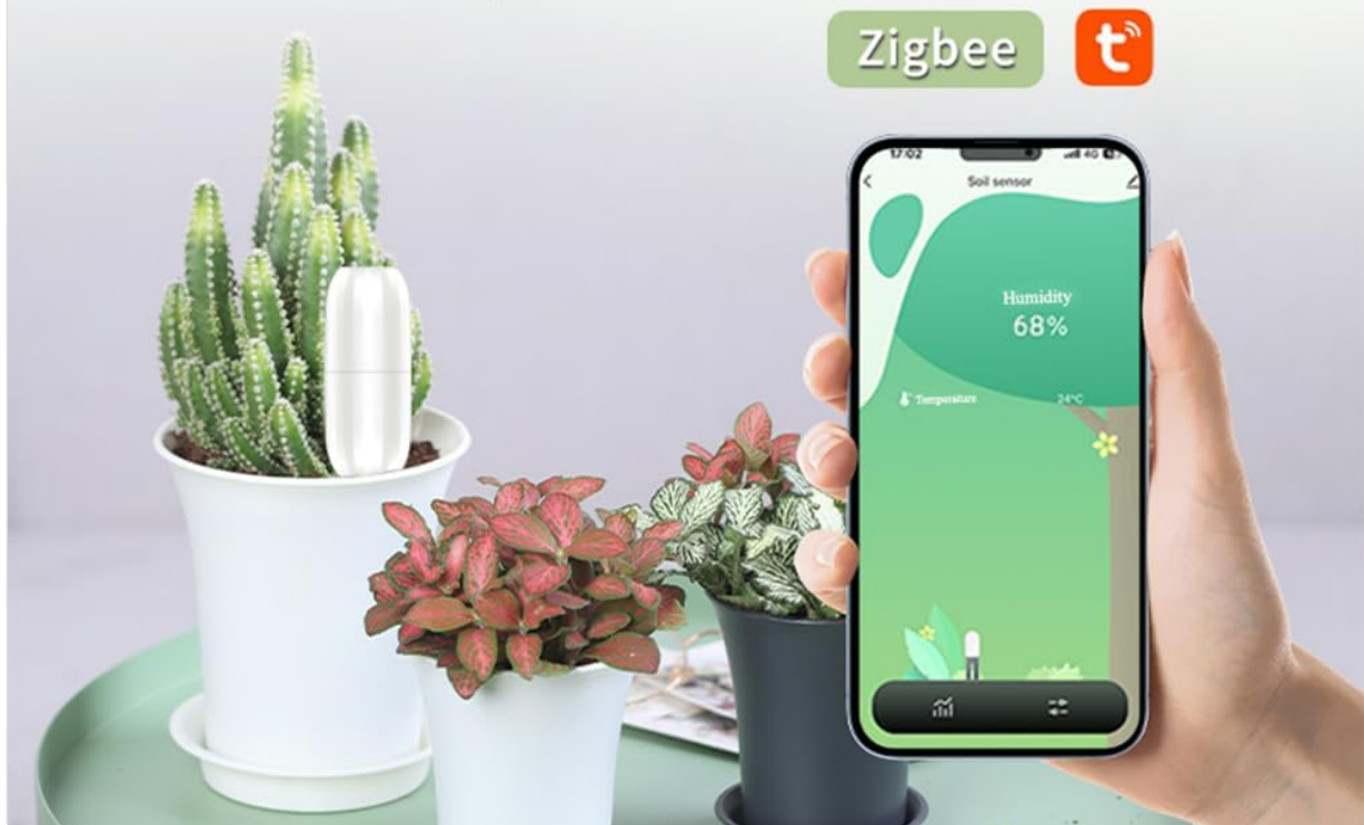
Figure 4: Screenshot of the mobile application displaying soil temperature and humidity data. This image illustrates how users can view real-time data and historical curves for effective plant monitoring.
