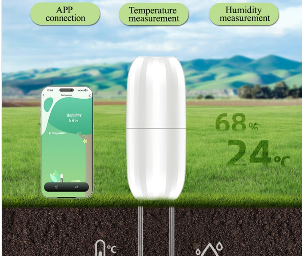
Figure 1: Haozee QT-SOIL Wireless Soil Moisture and Temperature Sensor. This image shows the overall design of the sensor, highlighting its wireless capabilities and dual measurement functions for temperature and humidity.
