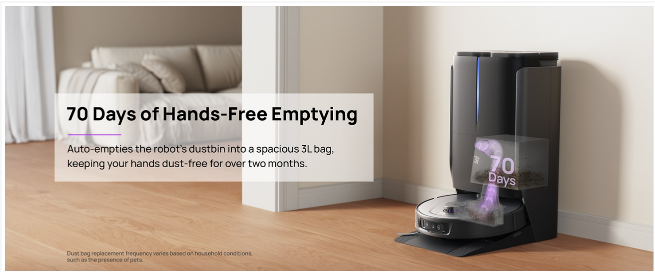
Figure 6.1: Automatic dustbin emptying at the base station.
