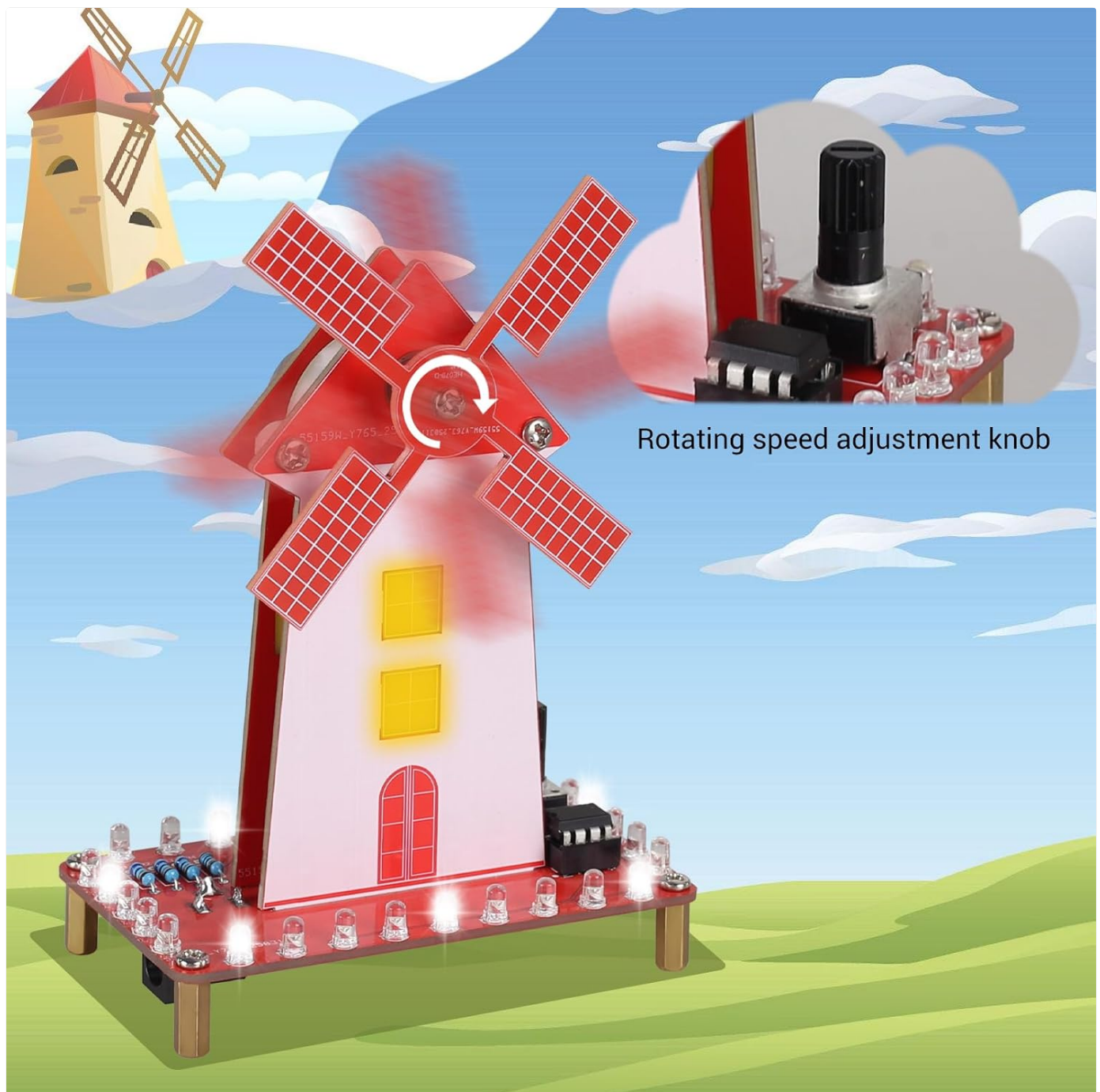
Close-up view of the windmill kit highlighting the rotating speed adjustment knob, used to control the blade rotation.
