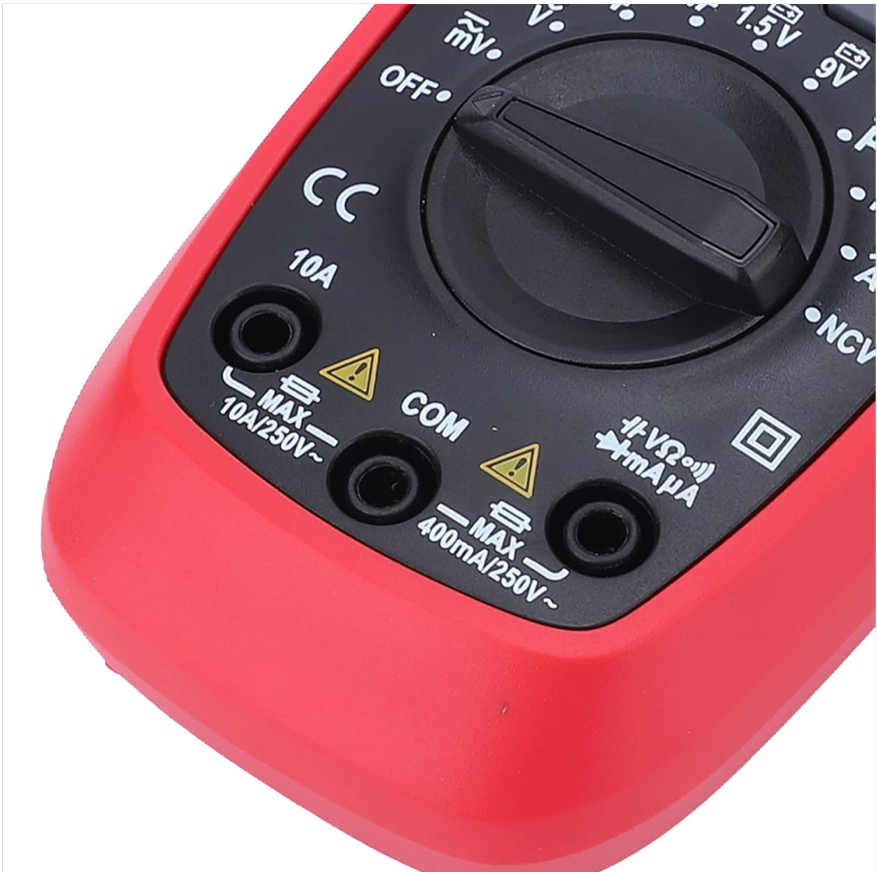
Image: Close-up of the multimeter's input jacks. The black COM jack, the red VΩmA jack, and the red 10A jack are visible.
