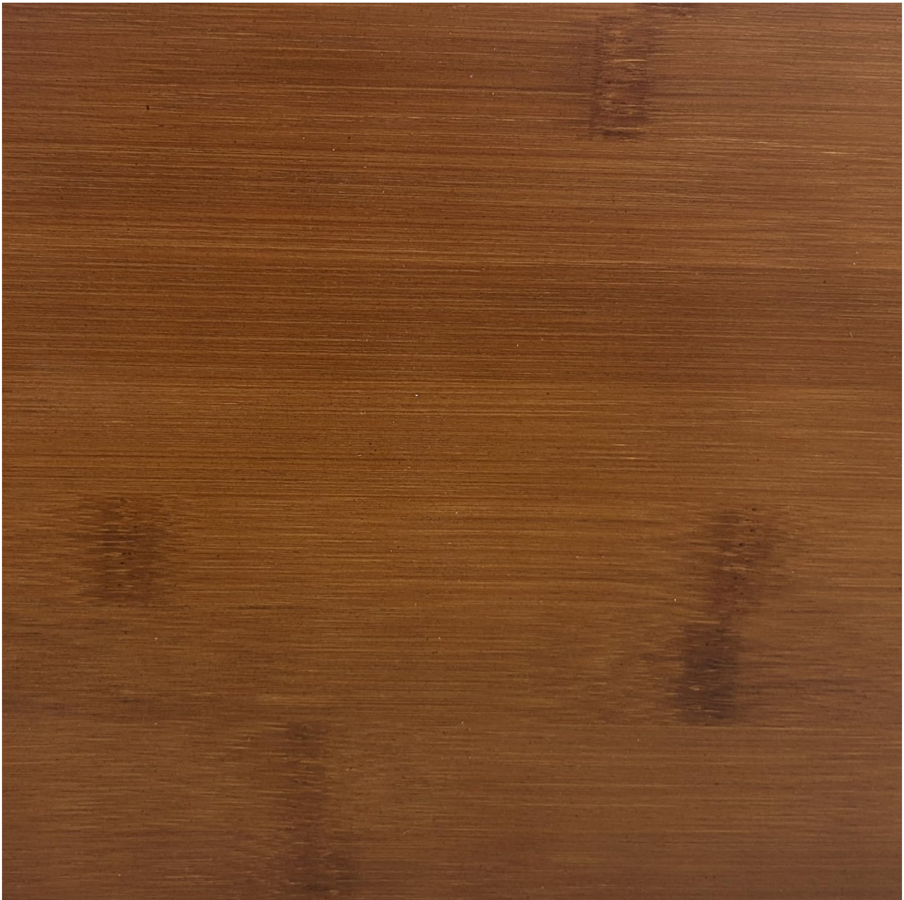
Image 6.1: Detail of the solid dry bamboo wood material.
